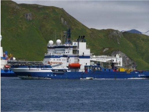
Ice management vessels such as the M/V *Fennica*, M/V *Nordica* (Photograph 2.2-3) or similar vessel will serve as ice management vessels in support of the drilling units. The ice management vessels will enter and exit the Chukchi Sea with or in advance of the drilling units. Ice management would be expected to occur at a distance of up to 20 mi (32 km) upwind or upcurrent of the drilling units, but ice reconnaissance may occur to a distance of 30 mi (48 km) or more.
