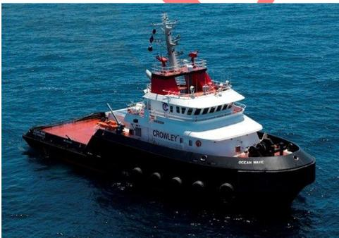
The drilling operations will require three ocean-going tugs such as the M/V *Ocean Wave* (Photograph 2.2-6) or similar vessels. Two tugs will serve as tow vessels / support tugs to the *Polar Pioneer* and remain near the drilling unit. One tug will also serve as a supply tug and will be moored in Kotzebue Sound when not supporting operations in the prospect.
