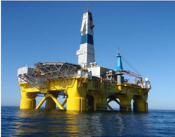
The *Polar Pioneer* (photo at left) is a non-selfpropelled, semi-submersible drilling unit capable of drilling in harsh environments. Its class notation is DNV 1A1 column stabilized drilling unit. It is a largely self-contained drilling unit that offers full accommodations for a crew of up to 114 persons, with quarters, galley, and sanitation facilities. General specifications for the *Polar Pioneer* are provided below in Table 2.2-1.
