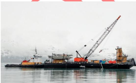
A nearshore OSR tug and barge such as the *Arctic Endeavor* or similar vessel (Photograph 2.2-12) and a tug (*Point Oliktok* or similar), will be staged in Goodhope Bay, Kotzebue Sound and would be mobilized in the event of a spill. It will carry a 47-ft (14-m) skimming vessel, three 34-ft (10-m) workboats, four mini-barges, and boom and duplex skimming units for nearshore recovery.
