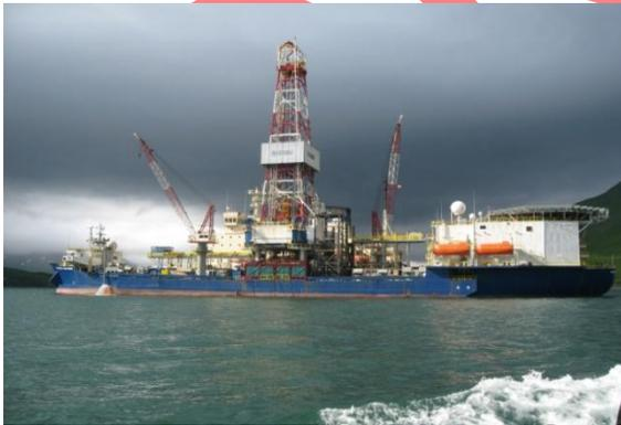
The *Discoverer* (photo to left) is an ice strengthened drillship and can mobilize under its own power. It is a largely self-contained drilling unit that offers full accommodations for a crew of up to 124 persons, with quarters, galley, and sanitation facilities. Specifications for the *Discoverer* are provided in Table 2.2-1.
