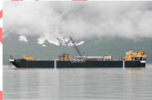
An offshore OSR tug and barge such as the *Klamath* (Photograph 2.2-11) or a similar vessel and a tug (*Guardman* or similar) (Photograph 2.2-11), will be staged offshore in the vicinity of the drilling unit. Together with the OSRV and the OST, there is sufficient containment, recovery, and storage capacity for the initial operational period in the event of a spill.
