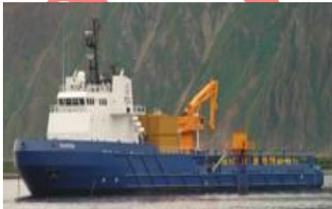
An OSRV such as the *Nanuq* (Photograph 2.2-9) will be staged offshore in the vicinity of the drilling units when any drilling unit is drilling in liquid hydrocarbon bearing zones such that it can immediately respond to a spill and provide containment, recovery, and storage for the initial operational period following a spill event.
