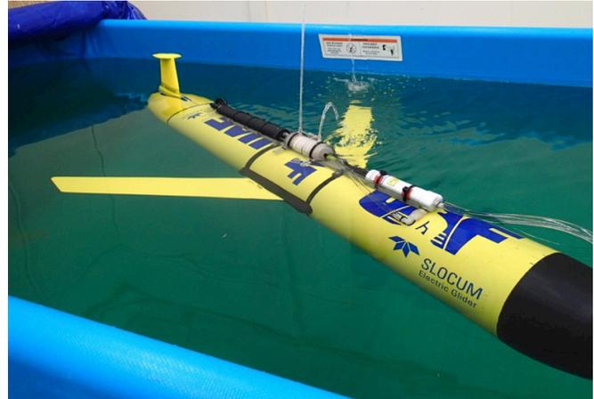
*Carbon glider in a tank at the UAF glider facilities during ballast testing.*
