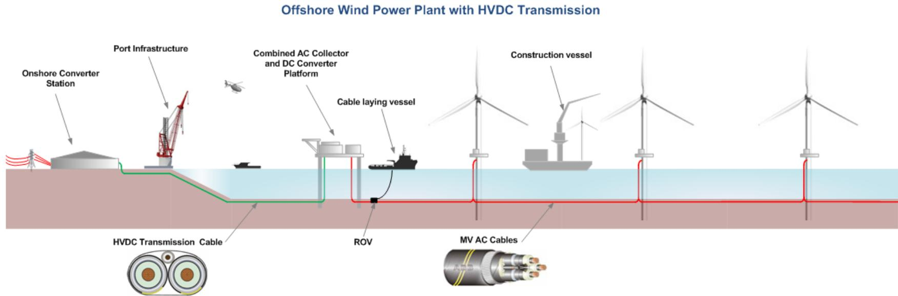
**Figure 4-1.** Diagram of OSW components (source: BOEM NREL 2014).
