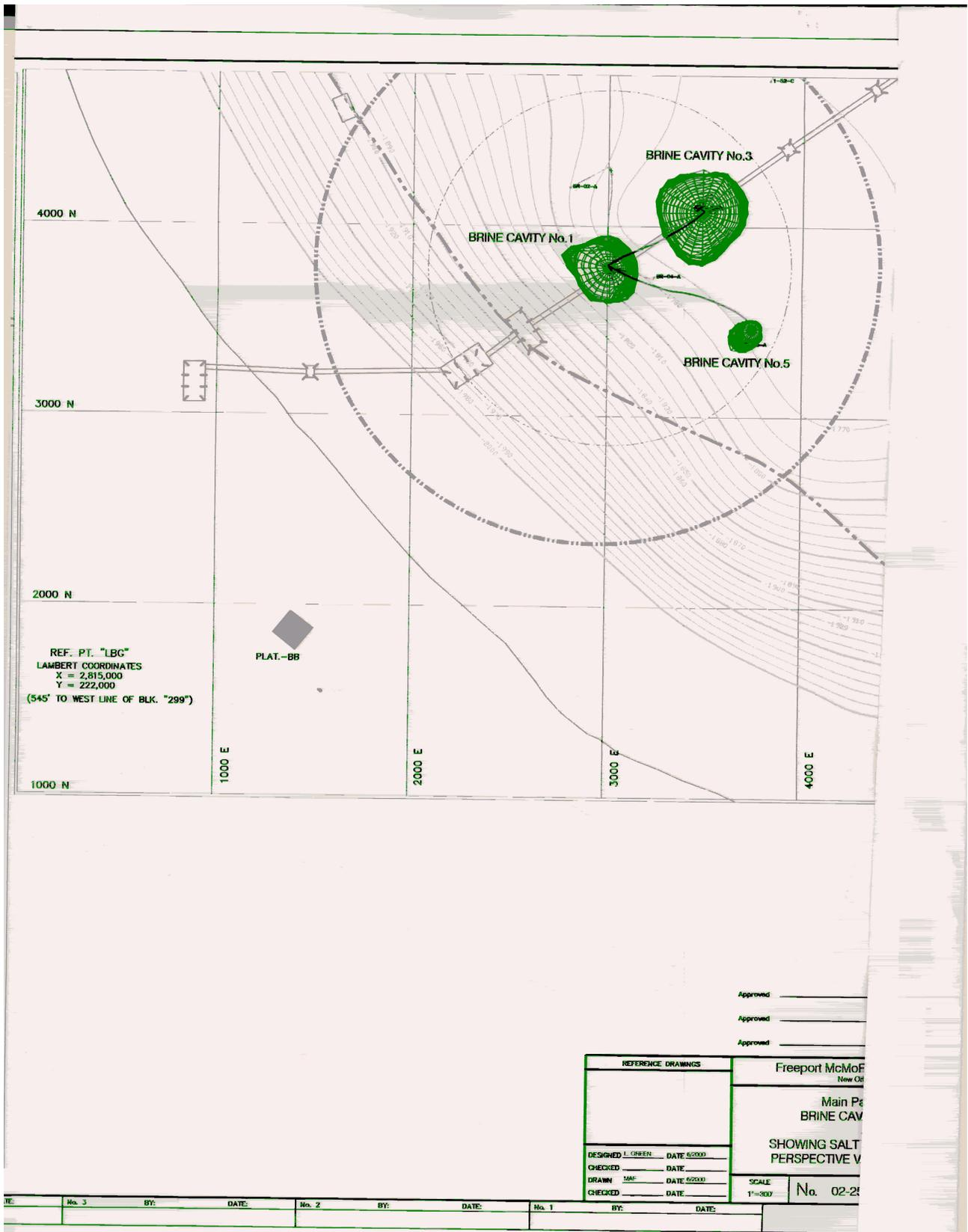
Figure B-3b. MP 299 plan view of Cavern Nos. 1, 3 and 5 in relationship to the platform complex.
