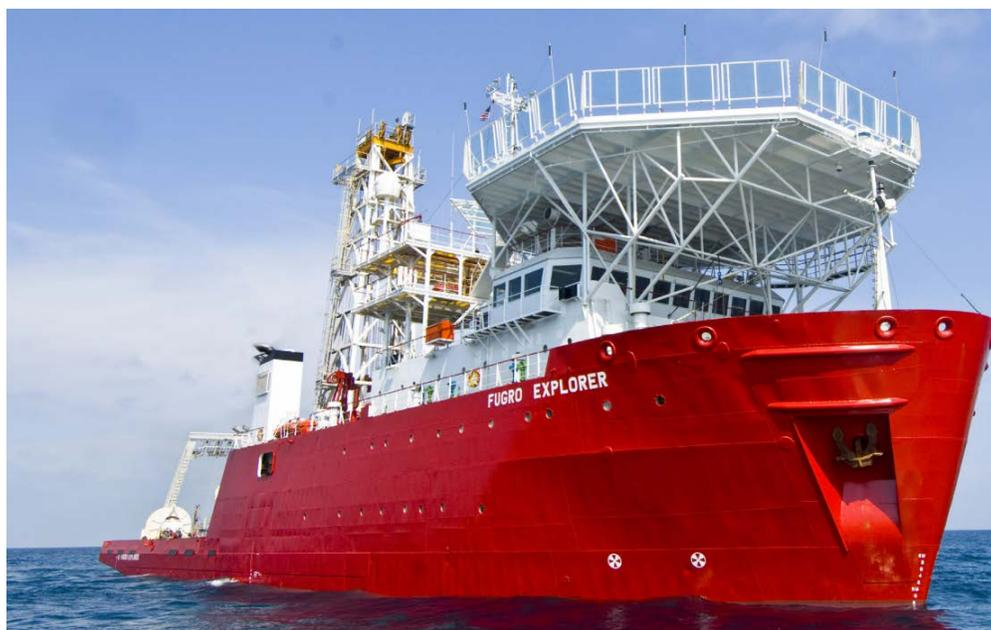
**Figure 3.1. An example of a dynamically-positioned vessel (Fugro Explorer)**
