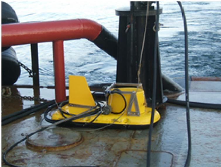
**Figure 6.13. Chirp sub-bottom profiler**
