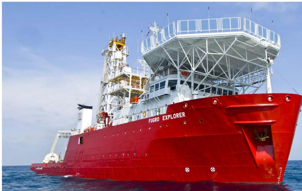
**Figure 6.1. An example of a dynamically-positioned vessel (Fugro Explorer)**
