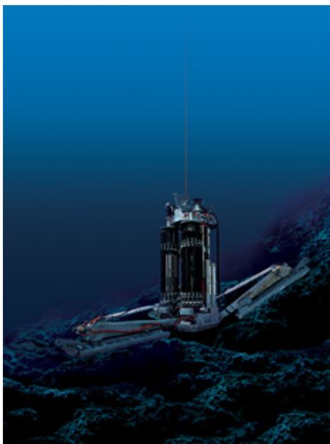
**Figure 3.4. Example of seafloor drill (Portable Remotely Operated Drill)**
