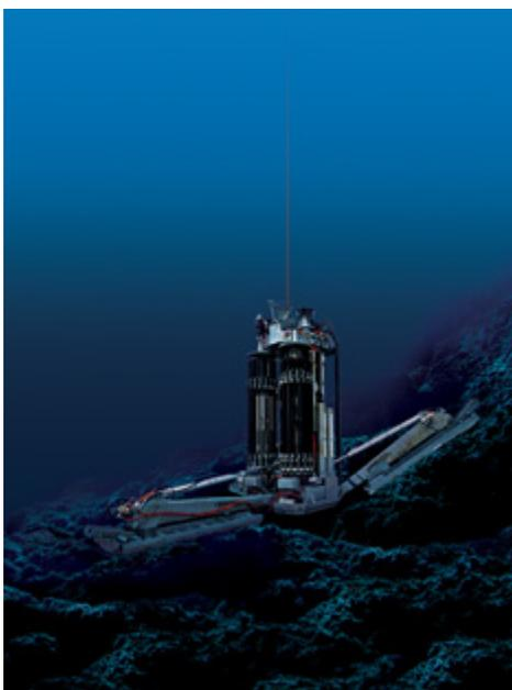
**Figure 6.4. Example of seafloor drill (Portable Remotely Operated Drill)**
