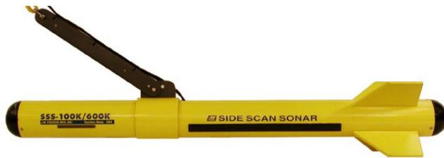
Photo 4. Sidescan Sonar Equipment (dual-frequency system) (USDOI, GS, 2013).
