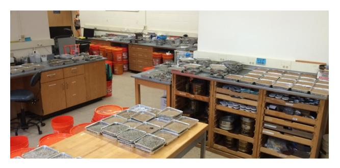
Figure 1. Picture from the University of Massachusetts Amherst sedimentology lab showing samples in pans in preparation for weighing and sieving for the greater than 4 mm fraction.
