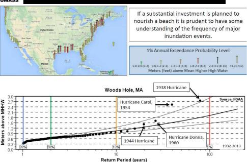
Figure showing how the magnitude of low frequency inundation events seemingly produces higher storm surges than expected.
