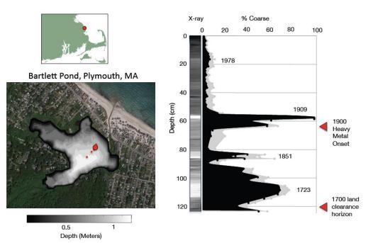
Figure showing results of x-ray scan and % coarse sand on BAP6 from Bartlett Pond, Plymouth, MA. Percent coarse sand on core BAP6 (left) showing sand peaks associated with storm events. Lead and onset of land clearing help constrain the age model for each core. Bright sections in x-ray scan represent sandier storm event layers (from Woodruff et al., 2015).
