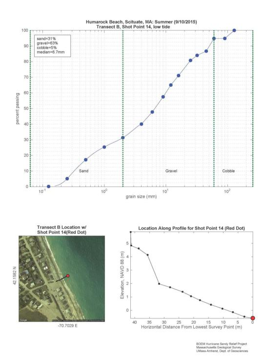
Figure 1. Example of grain size distribution plot (top) from Transect B, low tide sample in summer 2015 collected at Humarock Beach, Scituate, Massachusetts. Also shown is the location of the sample on the transect (lower left) and location of sample along beach profile (lower right).
