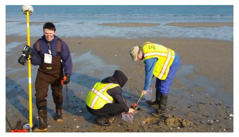
Figure 1. Example of sample collection. This sample collected at mid tide at Revere Beach in March 2016. Taking a gallon size sample.
