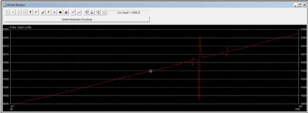
Figure 2-2. Real time graphical data trace of raw gamma values versus distance along a trackline.
