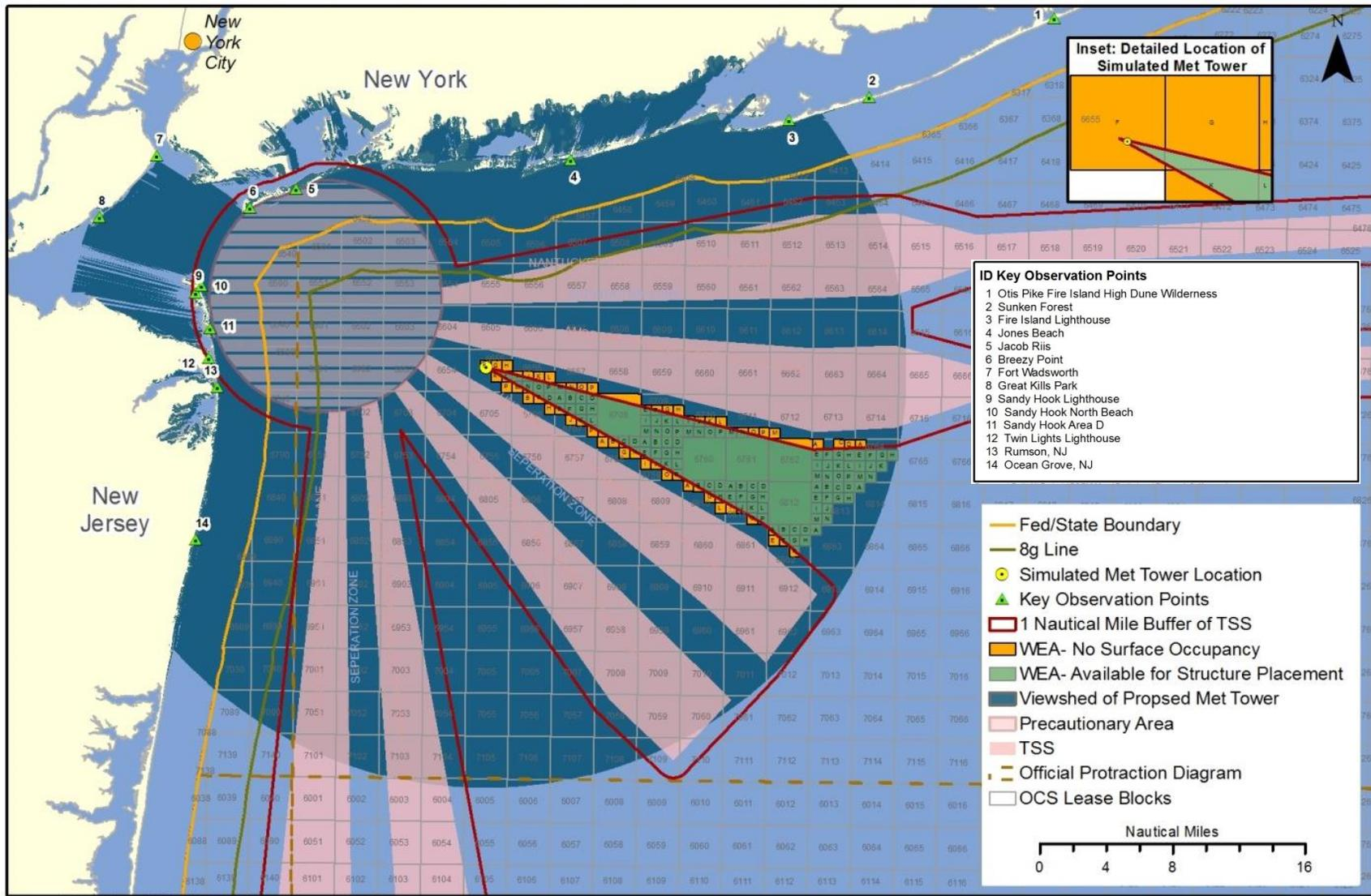
Figure 4-23 Meteorological Tower Viewshed and Key Observation Points
