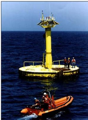
**Figure 3-5(a) 10-Meter Discus-Shaped Hull Buoy**
