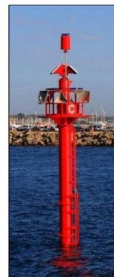
**Figure 3-5(c) Spar Buoy**
