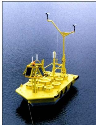
**Figure 3-5(b) 6-Meter Boat-Shaped Hull Buoy**
