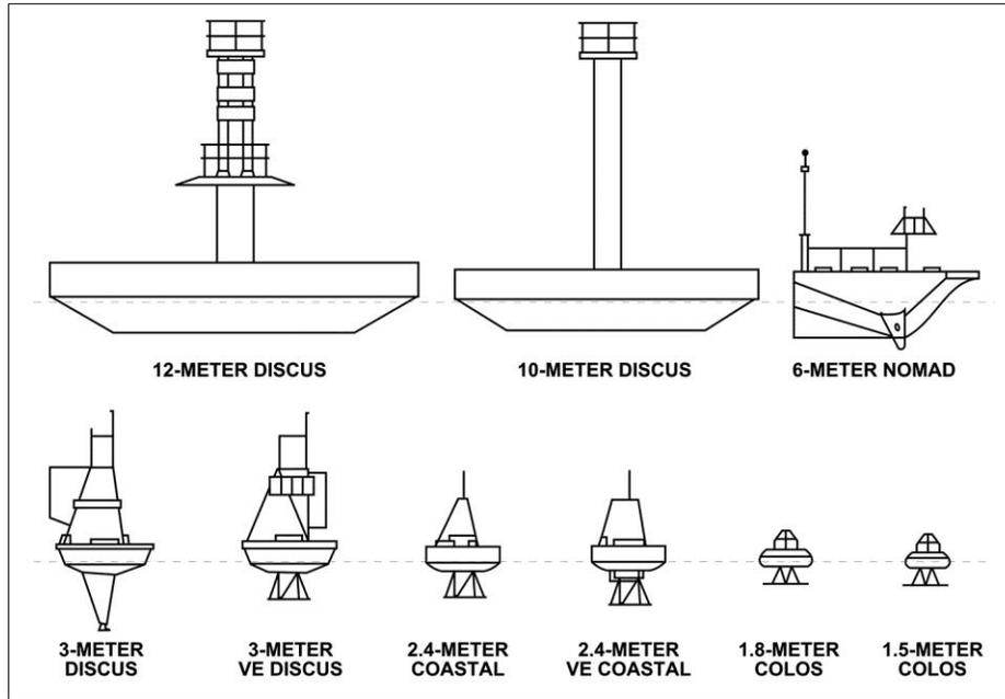
**Figure 3-4 Buoy Schematic**
