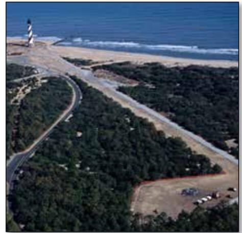
By 1999, the Cape Hatteras lighthouse (upper left) was less than 200 feet from shore and had to be relocated to an inland site (lower right). The historic move illustrates one of the ways Interior is adapting to the dynamic nature of barrier islands and reducing vulnerability to sea-level rise. Photo credit: NPS.
