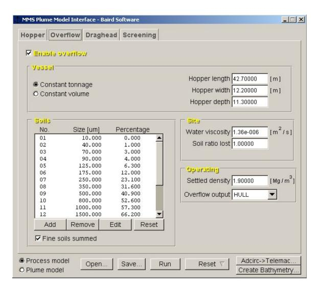
In this menu, specifics related to the hopper dimensions, the settled density within the hopper and the in-situ grain size curve are entered. The user can select either a *constant tonnage* system or a *constant volume* system.
