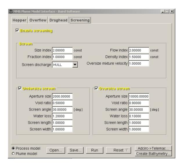
Undersize and oversize screening of the aggregate can be enabled by means of the various checkboxes. Screen dimensions and other screening-related properties are entered in this menu.
