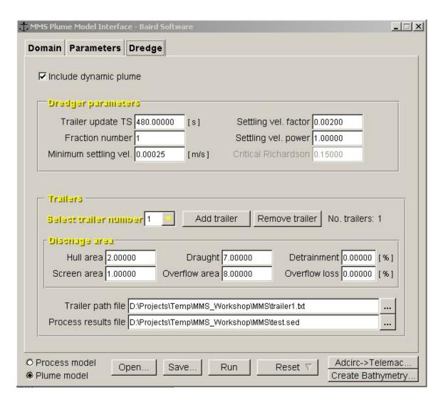
On this menu, the number and characteristics of each dredger (up to 10 in total) are entered including the grain (Fraction Number) size to be simulated, the dredger path, and overspill data such as discharge and mass rates, which are determined from the process model.
