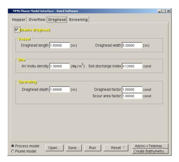
Draghead effects can be enabled by means of the checkbox. If it is enabled, the dimensions of the draghead and various other draghead properties must be entered.
