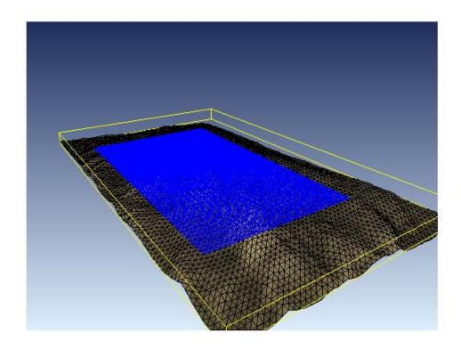
**FIGURE 2.** The Plume Model Rectangular Grid (in blue) Shown Embedded in the Larger ADCIRC Grid (in black)
