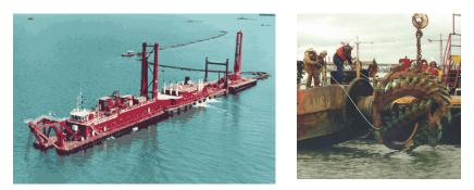
Figure 4. Great Lakes Cutter Suction Dredge California (left) and CutterHead (right) (Courtesy of Great Lakes Dredge & Dock)
