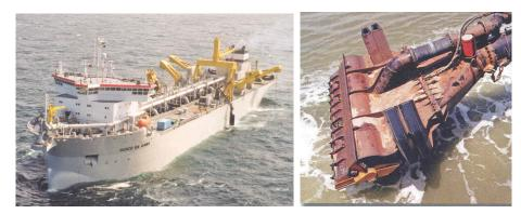
Figure 1. Jen de Nul's Vasco de Gamma (left) and Typical Draghead (right) (Courtesy of Jen de Nul)
