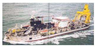
Figure 3. Self Propelled Cutter Suction Dredge JFJ de Nul (Courtesy of Jen de Nul)
