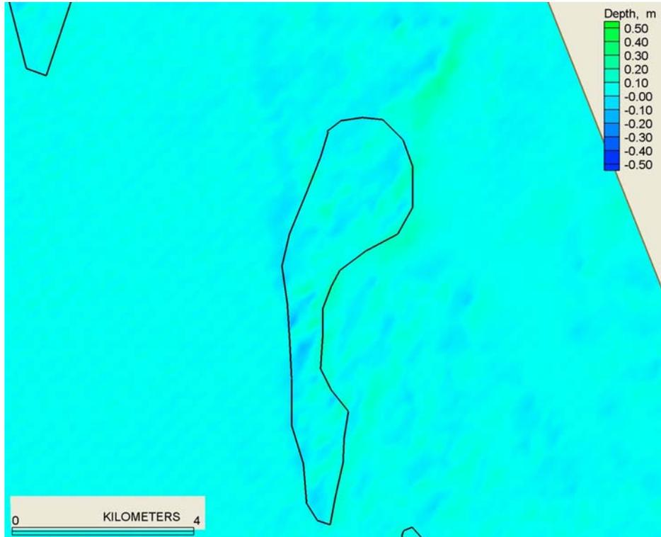
**Figure 4-49. Net predicted topographic change over the crest of the A9 model domain after two years of simulation. Maximum changes were +/- 25 cm (0.8 ft.).**
