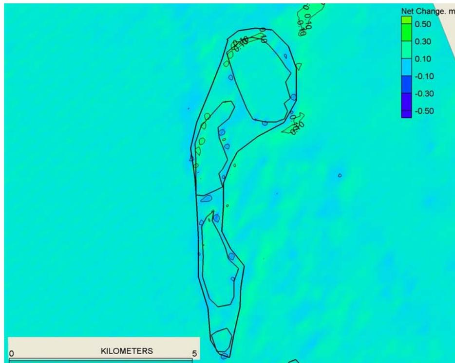
**Figure 4-50. Net predicted topographic change over the crest of the A9 model domain after two years of simulation with multiple borrow cuts (Case 6).**
