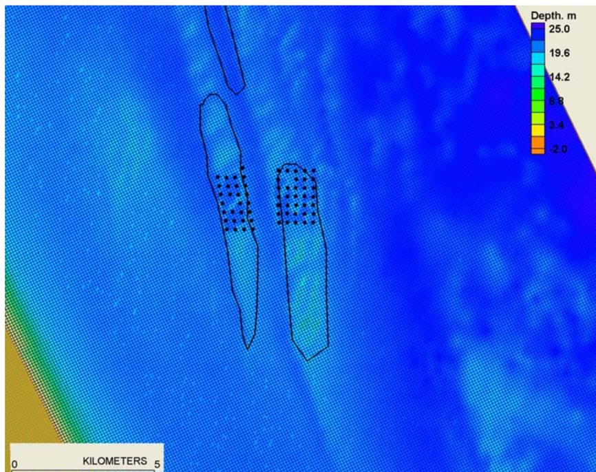
**Figure 4-12. Location of single borrow cuts in the B12 and B11 shoals based on geotechnical information developed by Volusia County, Florida. Vibracore locations marked with black circles.**
