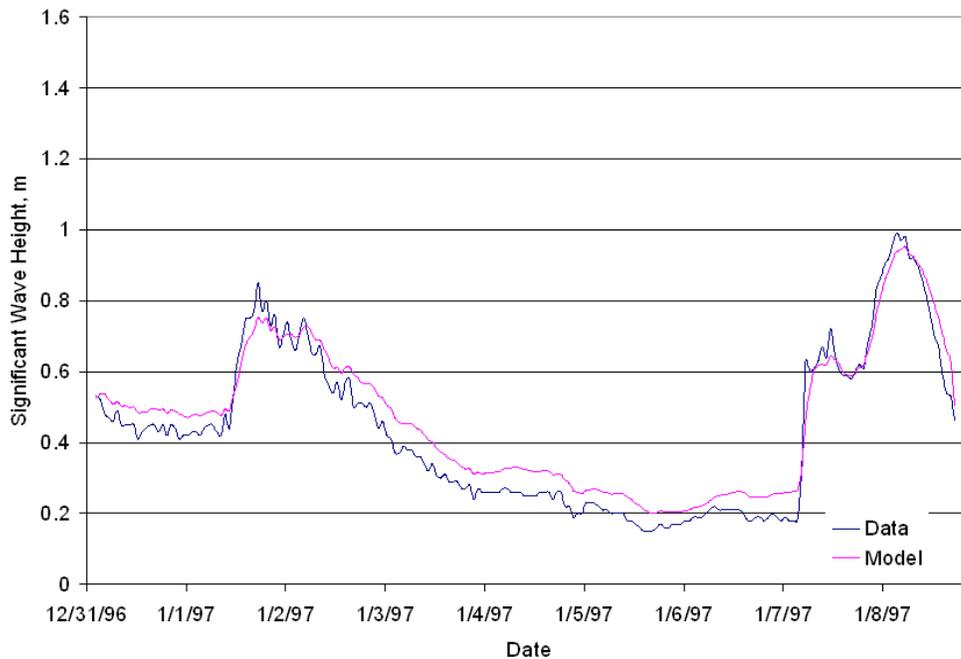
**Figure 4-6. Comparison between modeled and measured significant wave heights for the first 10 days of 1997. Gauge location is shown in Figure 4-2.**
