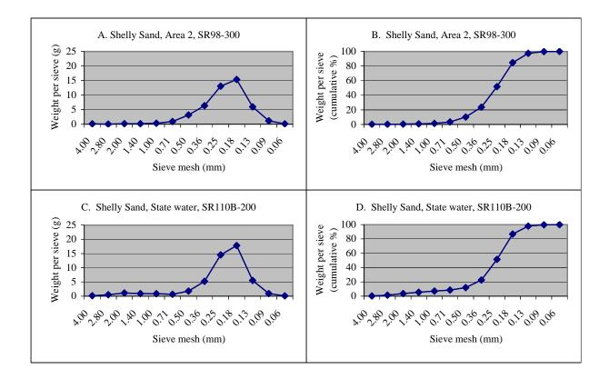
Figure 22. Frequency and cumulative frequency curves of Shelly Sand samples. (A) Area 2, SR-98-300, frequency curve; (B) Area 2, SR-98-300, cumulative frequency curve; (C) State waters, SR-110B-200, frequency curve; (D) State waters, SR-110B-200, cumulative
