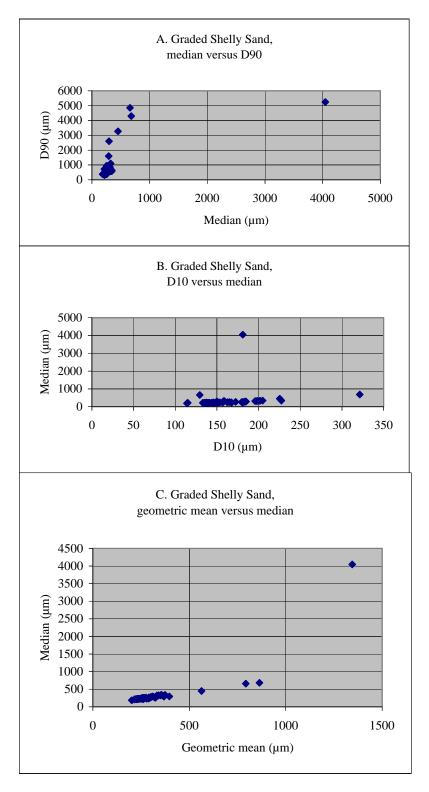
Figure 17. Bivariate comparisons of particle-size parameters for the Graded Shelly Sand lithofacies. (A) median particle size versus D90 (size greater than that of 90 percent of particles), (B) D10 versus median particle size, (C) geometric mean versus median particle size.
