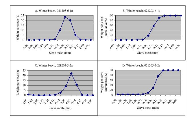
Figure 6. Frequency and cumulative frequency curves of winter beach sand samples. (A) 021203-06-1a, frequency curve; (B) 021203-6-1a, cumulative frequency curve; (C) 021203-3-2a, frequency curve; (D) 021203-3-2a, cumulative frequency curve.
