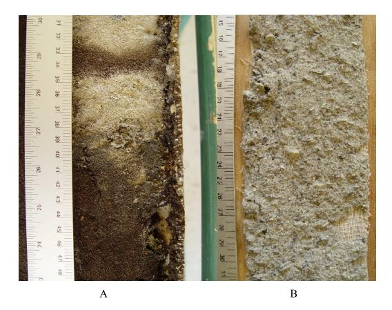
Figure 9. Photographs of vibracores including tentatively identified echinoid burrows *Subphyllochorda*. (A) Vibracore SR-102A with possible echinoid burrow at about 34.5-39 cm downcore. (B) Peel of vibracore SR-7B with probable but subtle echinoid burrows at about 162-167 cm downcore (corresponding to 17-22 cm in photograph).
