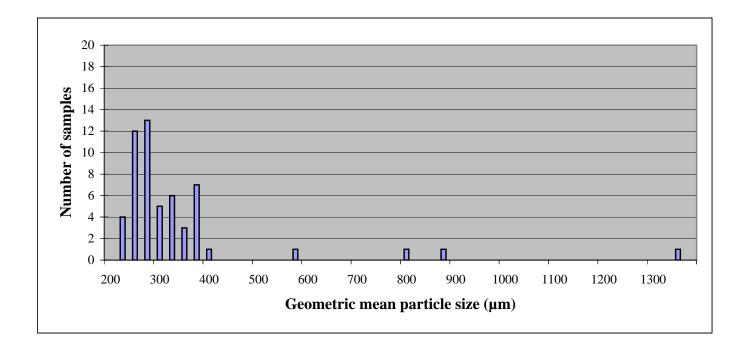
Figure 16. Histogram of geometric mean particle sizes of sieved samples from the Graded Shelly Sand lithofacies.
