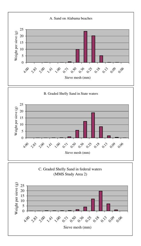
Figure 5. Histograms comparing particle-size distributions of representative samples of (A) Alabama beach sand, sample 021203-6-1a; (B) Graded Shelly Sand lithofacies in State waters, SR-109A -100; and (C) Graded Shelly Sand lithofacies in federal waters (MMS Study Area 2), SR-101A-15.
