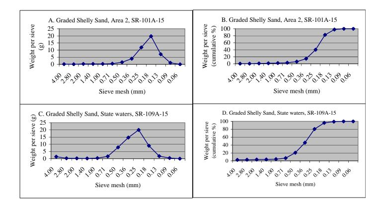
Figure 19. Frequency and cumulative frequency curves of Graded Shelly Sand samples. (A) Area 2, SR101A-15, frequency curve; (B) Area 2, SR101A-15, cumulative frequency curve; (C) State waters, SR109A-15, frequency curve; (D) State waters, SR109A-15, cumulative frequency curve.
