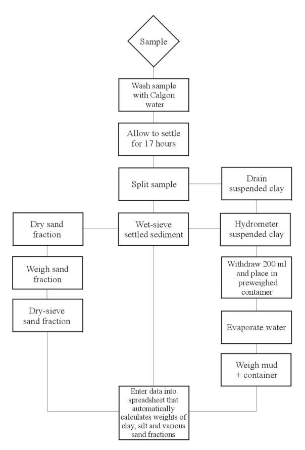
Figure 3. Flow chart for particle-size analysis.
