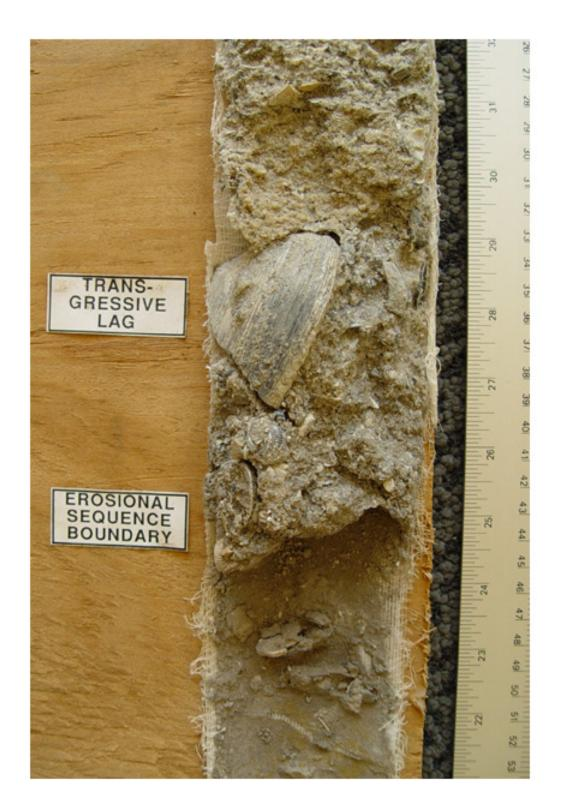
Figure 13. Coarse shell lag at base of graded layer in the Graded Shelly Sand lithofacies, vibracore SR-31. Centimeter scale (right) indicates depth downcore.
