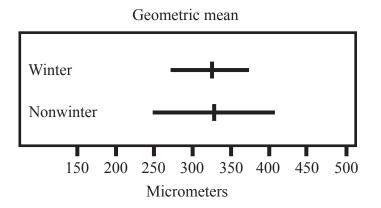
Figure 7. Means and standard deviations of geometric means of winter (n = 7) and nonwinter (n = 70) sieve data from Alabama beaches.
