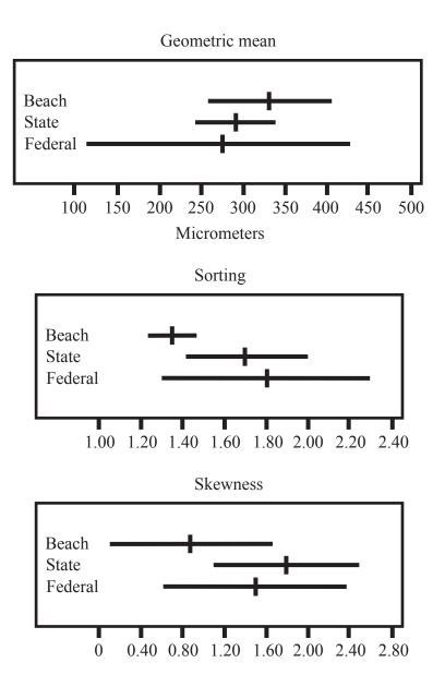
Figure 4. Means and standard deviations of three moment measures of Alabama beach sand, sand in state waters, and sand in federal waters.
