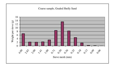
Figure 15. Histogram of relatively coarse sample from Graded Shelly Sand lithofacies, vibracore SR-23-bg.
