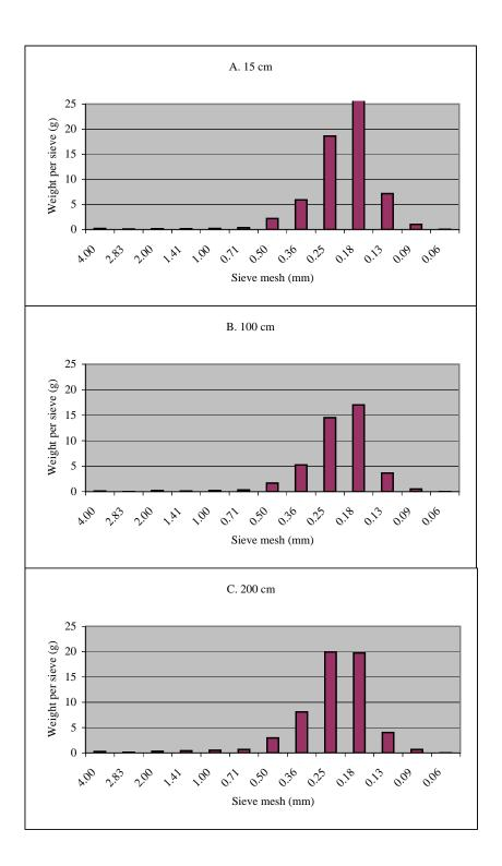
Figure 18. Subtle normal grading in sediment particle size within a graded layer (vibracore SR-113) at (A) 15 cm, (B) 100 cm, and (C) 200 cm downcore.
