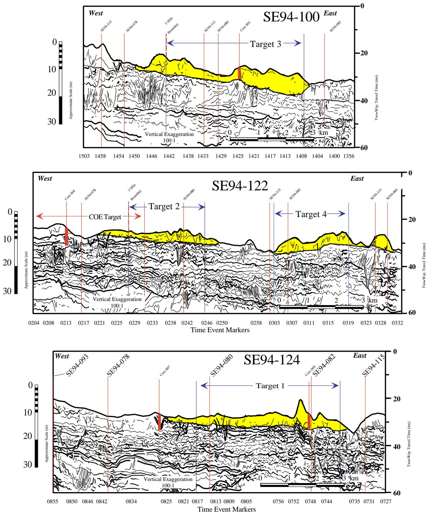
Figure 2. Example seismic sections crossing prospective sand resource areas (targets). See Figure 1 for location information. The seismically transparent unit is shown in yellow.
