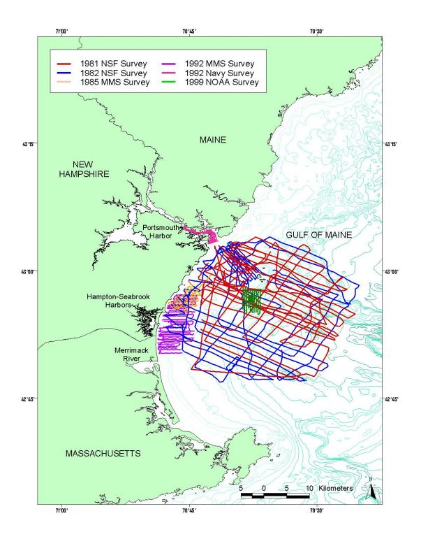
Figure 2. Seismic tracks from previous studies conducted by the University of New Hampshire.
