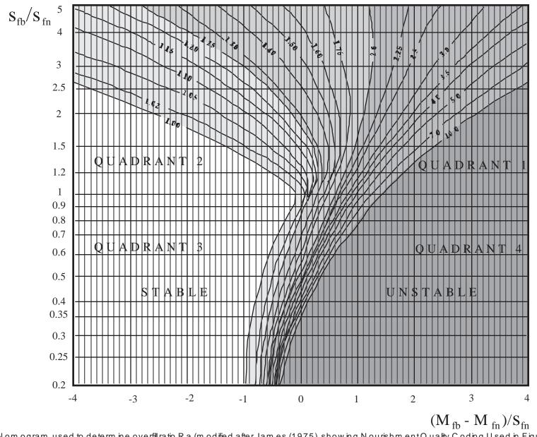
Figure 14: Nom ogram used to determ ine overfill ratio R a (modified after James (1975). showing Nourishment Quality Coding Used in Figures 13 and 18. Overfill ratios greater than 1.25 are generally considered unstable and unsuitable as beach fill material.
