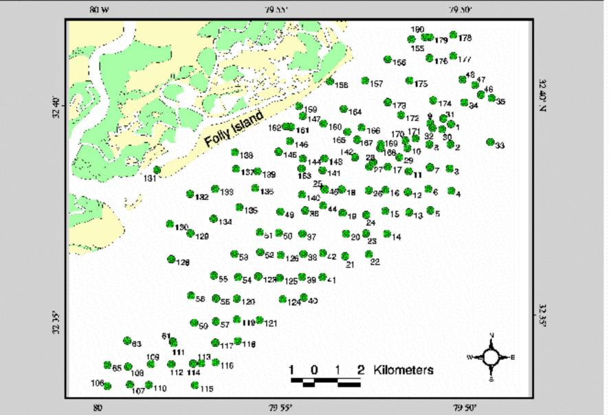
Figure 7. Surficial sediment sample location map for the inner shelf off Folly Island, South Carolina. Sediment texural parameters are provided in Appendix 1.
