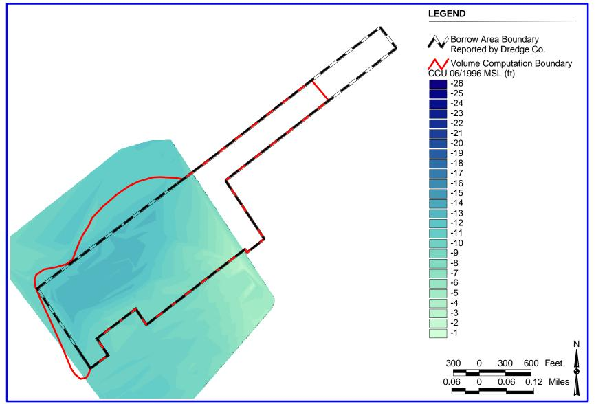
Figure 20. Joiner Bank borrow site with bathymetric data from the 1996 post-construction survey conducted by Coastal Carolina University.
