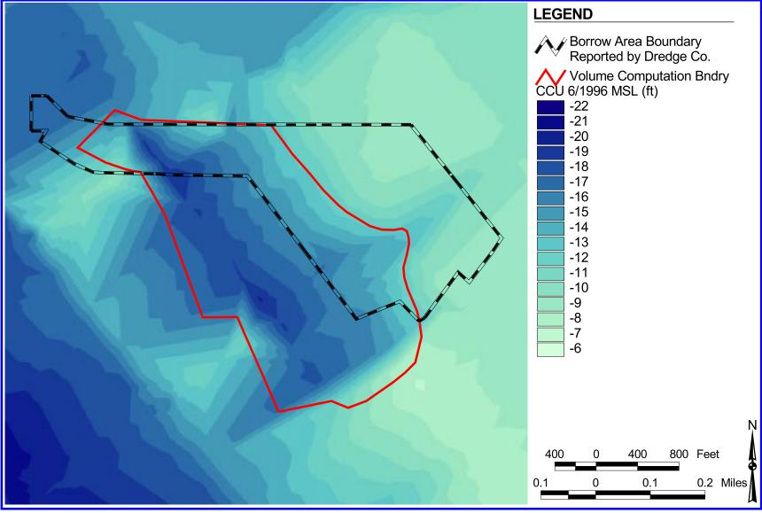
Figure 22. Gaskin Banks borrow site with bathymetric data from the 1994 post construction survey provided by Olsen Associates, Inc.
