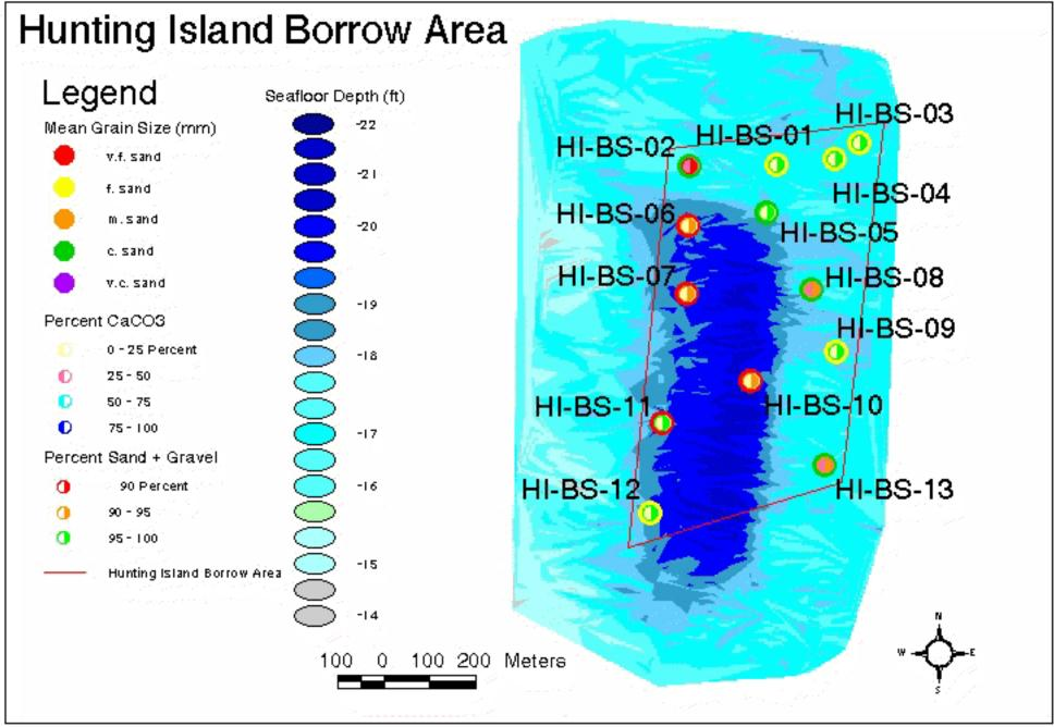
Figure 28. Location of stations sampled at the Hunting Island borrow site by Coastal Carolina University during the 1996 survey, with summaly information on sediment gain size and composition overlaid on the 1996 bathymetry data.
