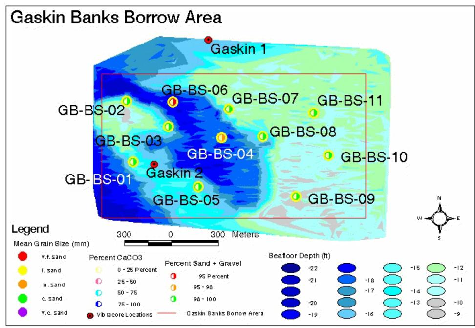
Figure 26. Location of stations samples at the Gaskin Banks borrowsite by Coastal Carolina University duing the 1996 survey, with summary information on sediment grain size and composition overlaid on the 1996 bathymetry data.
