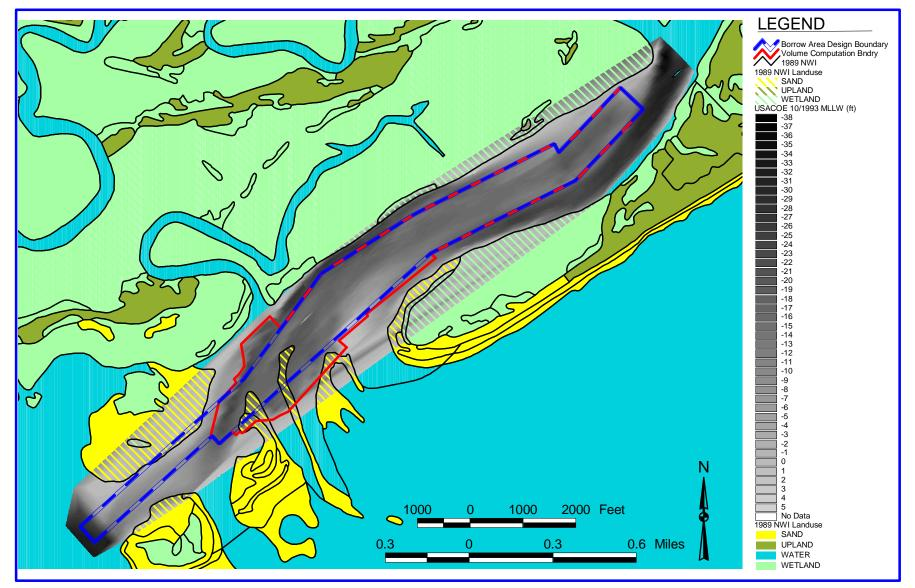
Figure 14. Folly River borrow site with bathymetric data from the USACOE post-construction survey (10/93).
