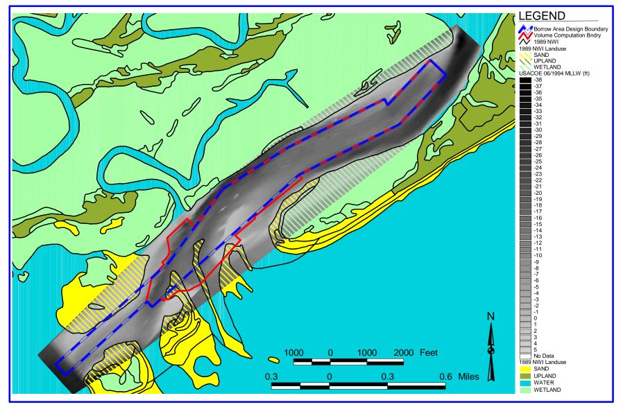
Figure 15. Folly River borrow site with bathymetric data from the USACOE post-construction survey (6/94).
