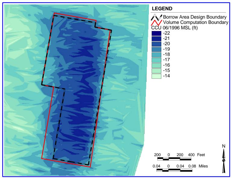
Figure 27. Hunting Island borrow site with bathymetric data from the 1996 post-construction survey conducted by Coastal Carolina University.
