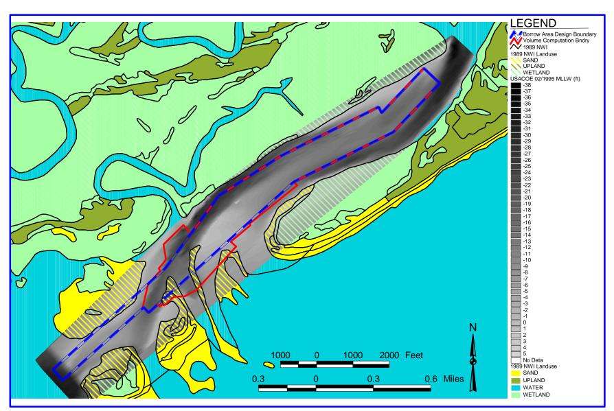
Figure 16. Folly River borrow site with bathymetric data from the USACOE post-construction survey (2/95).
