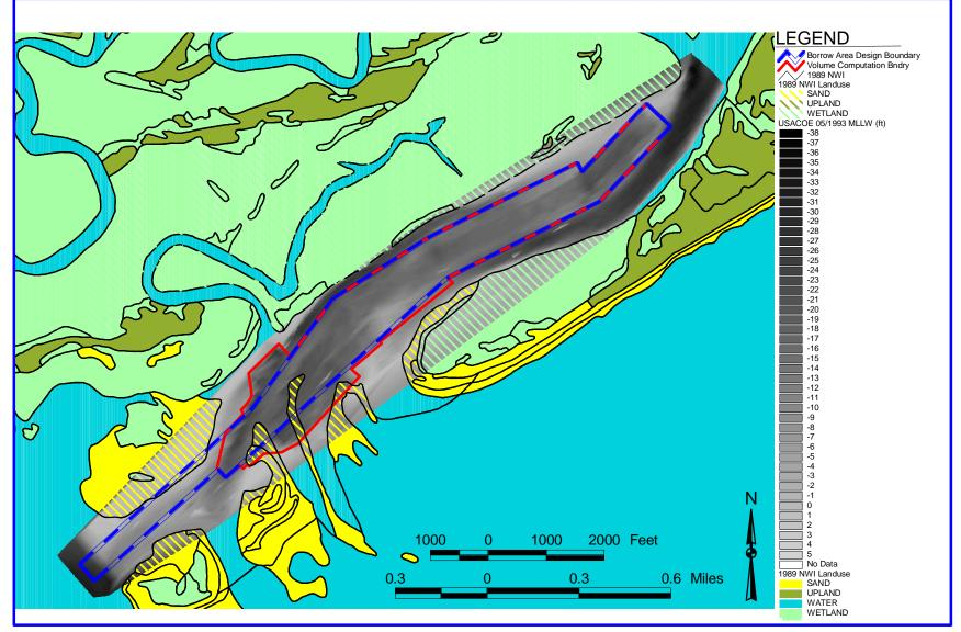
Figure 13. Folly River borrow site with bathymetric data from the USACOE post-construction survey (5/93).
