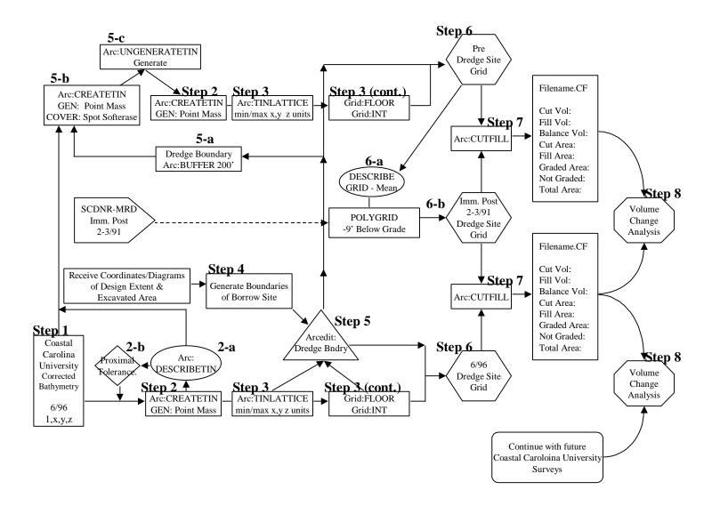
Figure 10. GIS Processing flowchart of the volume change analysis for the Hunting Island borrow site.
