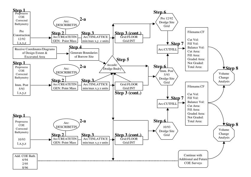
Figure 7. GIS Processing flowchart of the volume change analysis for the Folly River borrow site.
