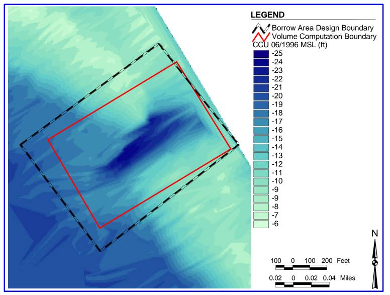
Figure 29. Edisto Island borrow site with bathymetric data from the 1996 post-construction survey conducted by Coastal Carolina University.
