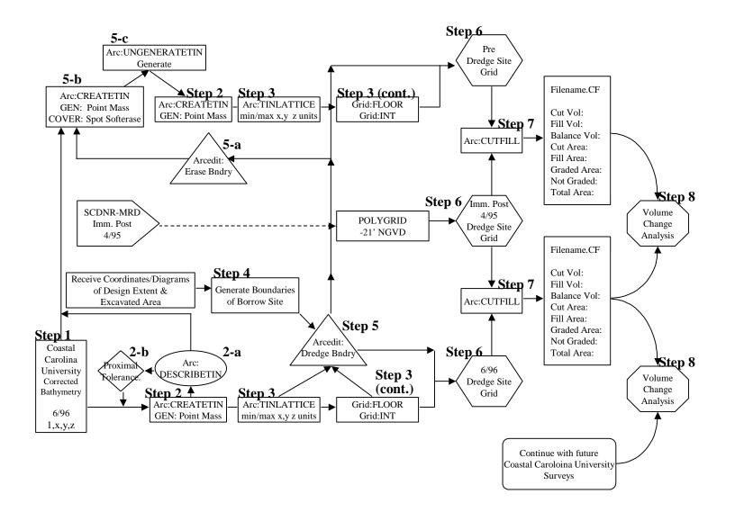
Figure 11. GIS Processing flowchart of the volume change analysis for the Edisto Island borrow site.
