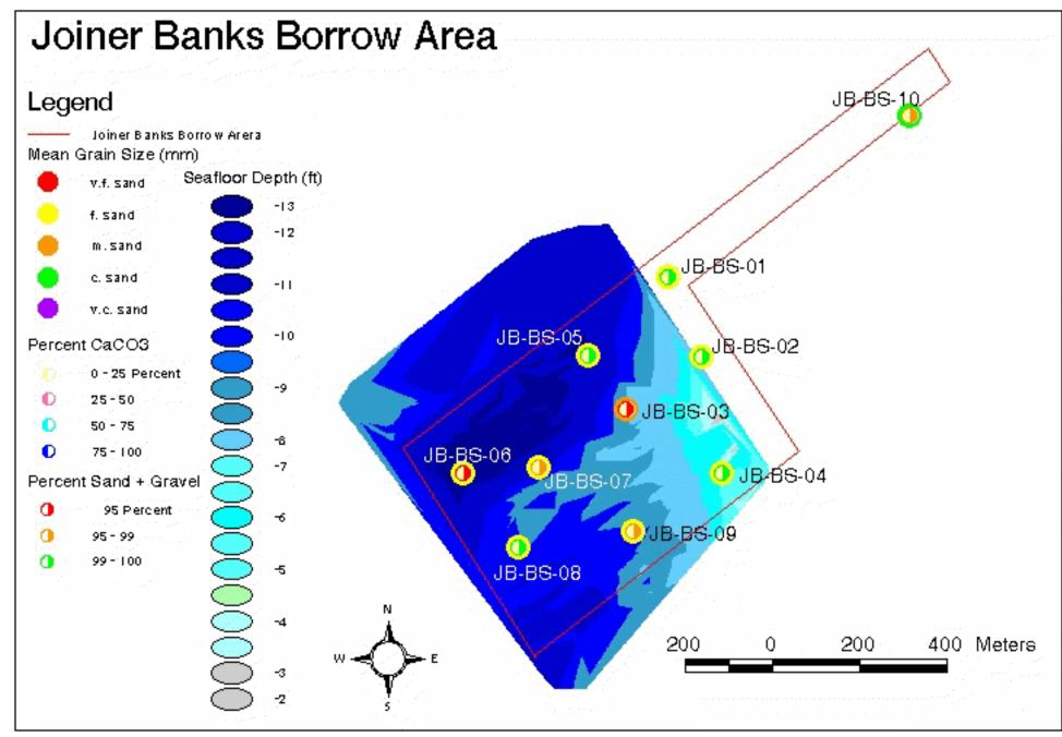
Figure 24. Location ofstations sampled at the Joiner Bark borrowsite by Coastal Carolina University during the 1996 survey, with summary information on sediment grain size and composition overlaid on the 1996 bathymetry data.
