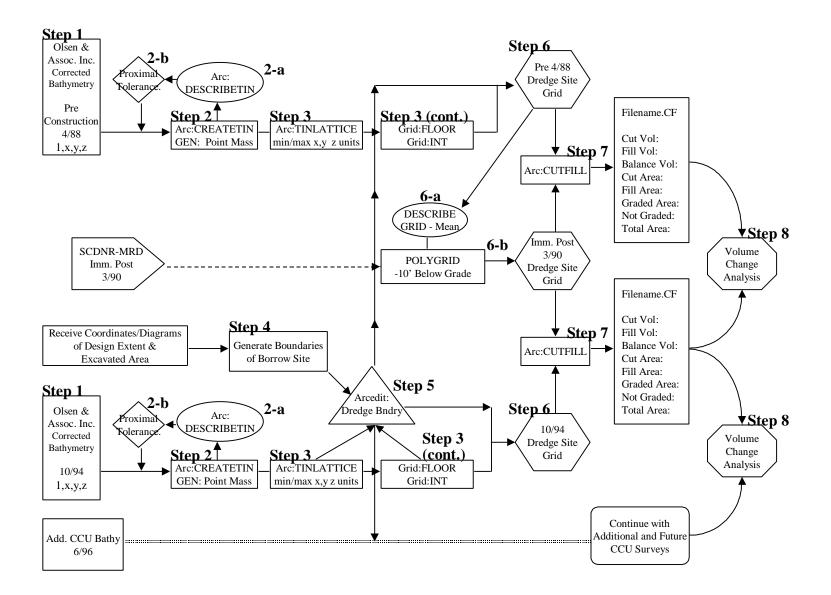
Figure 8. GIS Processing flowchart of the volume change analysis for the Joiner Bank (Hilton Head Island) borrow site.
