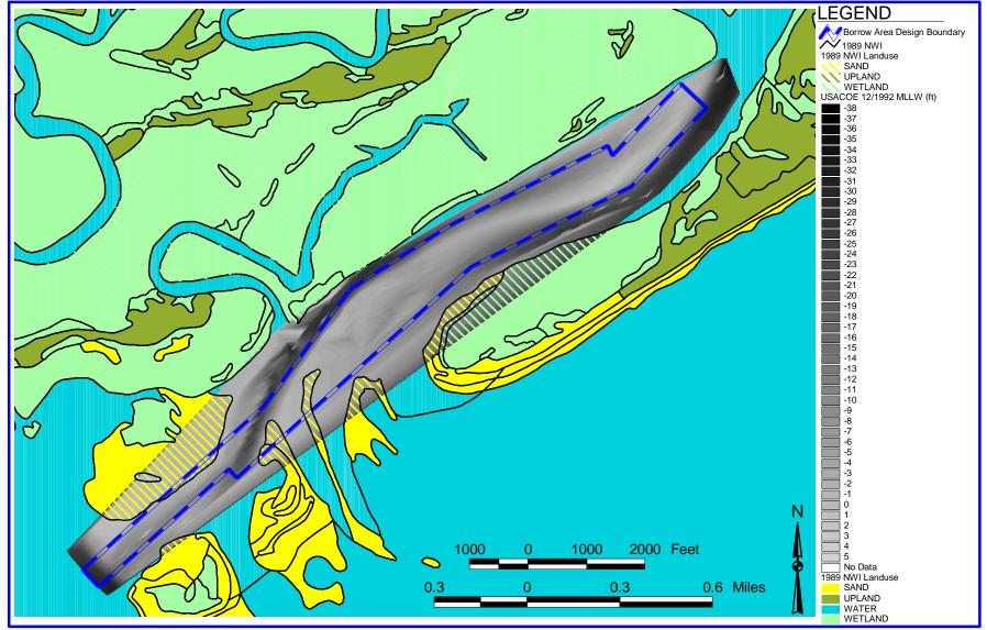
Figure 12. Folly River borrow site with bathymetric data from the USACOE pre-construction survey (12/92).
