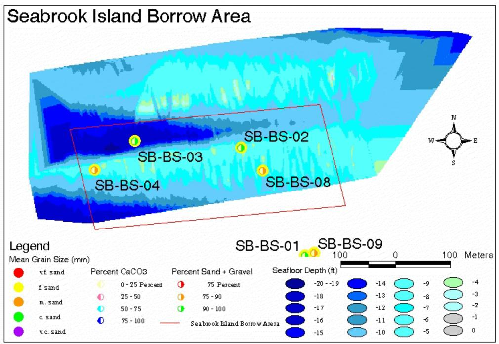
Figure 32. Location of stations sampled at the SeabrookIsland Borrow Site by Coastal Carolina University during the 1996 survey, with summary information on sediment grain size and composition overlaid on the 1996 bathymetry data.
