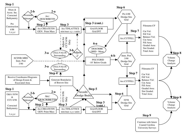
Figure 9. GIS processing flowchart of volume change analyses for the Gaskin Banks (Hilton Head Island) borrow site.
