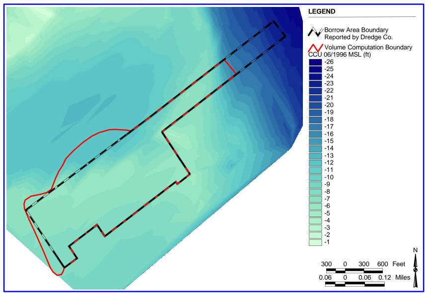
Figure 18. Joiner Bank borrow site with bathymetric data from the 1988 pre-construction survey provided by Olsen Associates, Inc.
