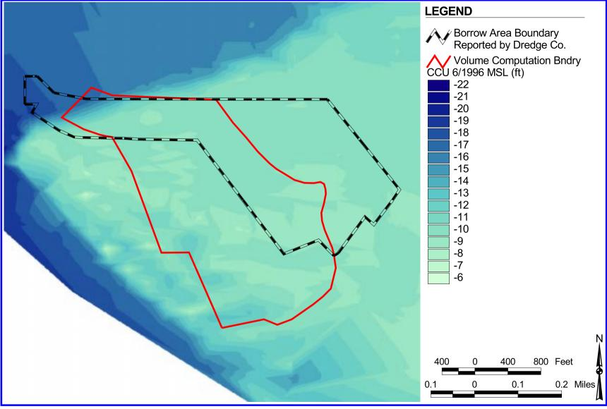
Figure 21. Gaskin Banks borrow site with bathymetric data from the 1988 pre-construction survey provided by Olsen Associates, Inc.
