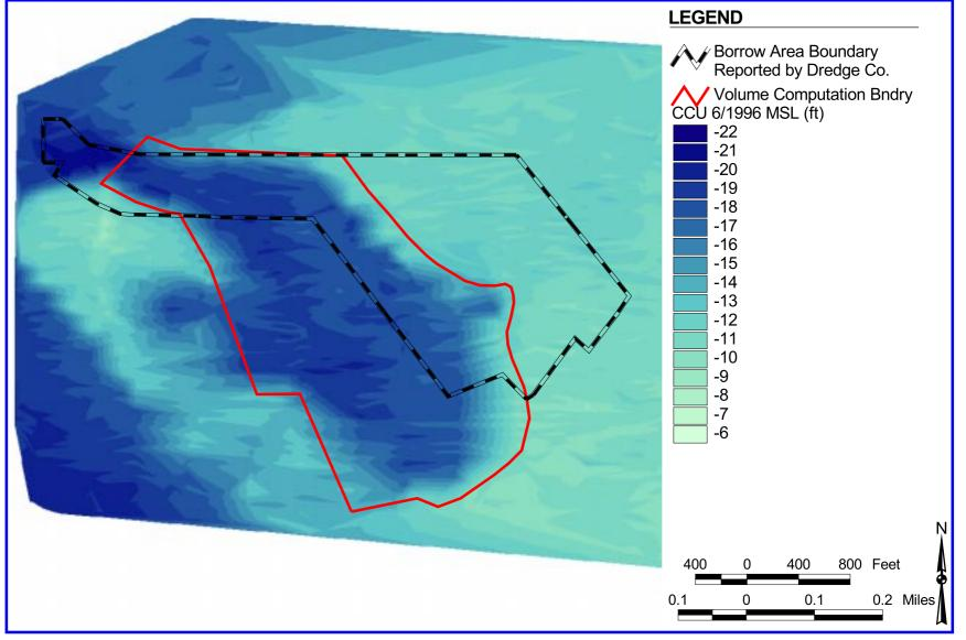
Figure 23. Gaskin Banks borrow site with bathymetric data from the 1996 post construction survey conducted by Coastal Carolina University.
