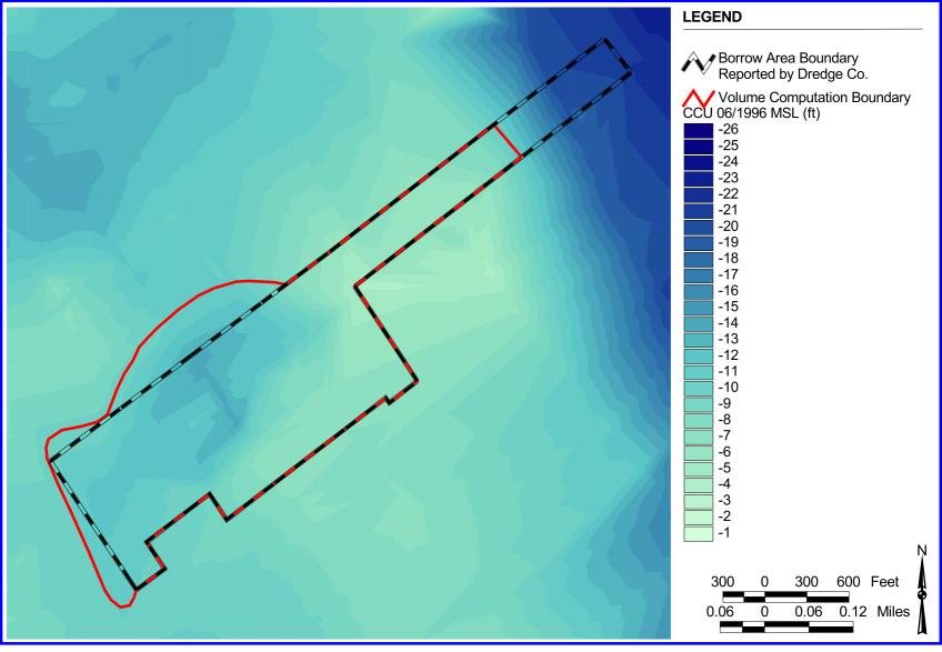
Figure 19. Joiner Bank borrow site with bathymetric data from the 1994 post-construction survey conducted by Coastal Carolina University.
