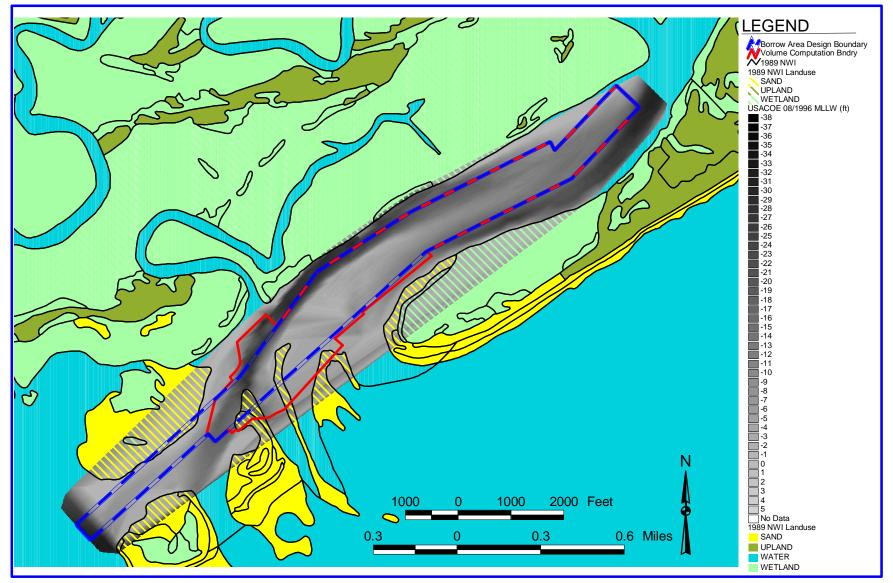
Figure 17. Folly River borrow site with bathymetric data from the USACOE post-construction survey (8/96).
