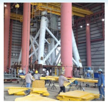
Workers at Gulf Island Fabrication built the steel jackets and decks for the first American offshore wind project.
