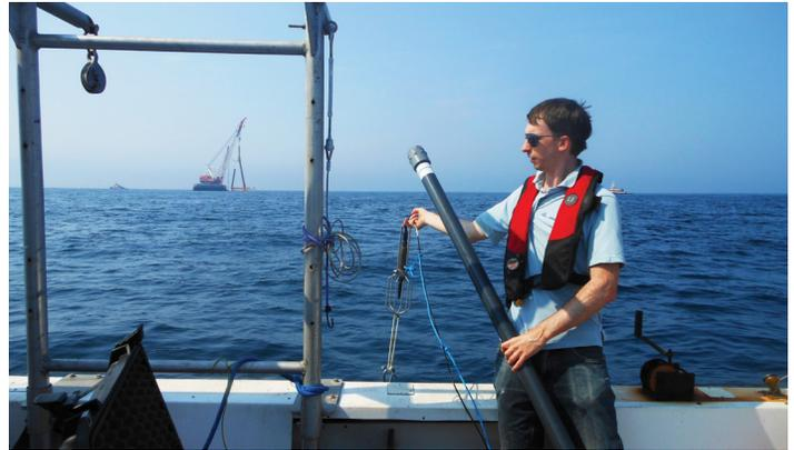
Deploying an acoustic monitor near the Block Island Wind Farm during the RODEO study.
