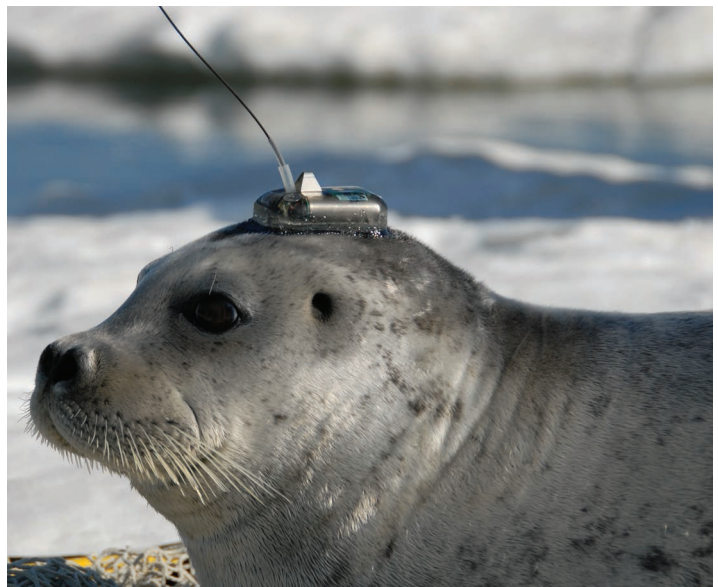
Adult bearded seal with a head-mounted Mk10 SDR in Kotzebue Sound, Alaska, in 2011. Photo by John Jansen, Alaska Fisheries Science Center, NOAA Fisheries
