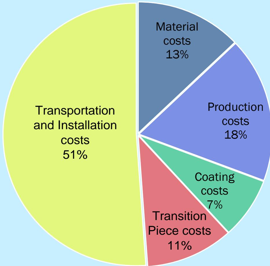
Jacket Cost Breakdown for 5 MW System
