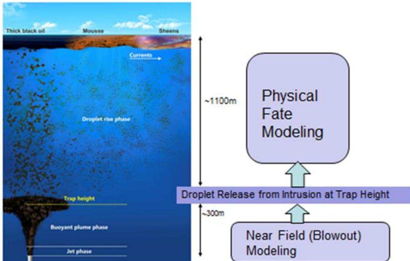
**Blowout Model (OILMAP-DEEP) simulates blowout plume dynamics for well blowouts, calculates the range of oil droplet sizes and provides inputs directly to the 3-D oil transport and fate model.**
