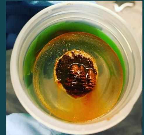
Corrosion products on carbon steel disk after 6 weeks in deep-sea water amended with oil
