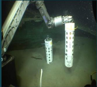
Biofilm recruitment experiments placed on seafloor by ROV
