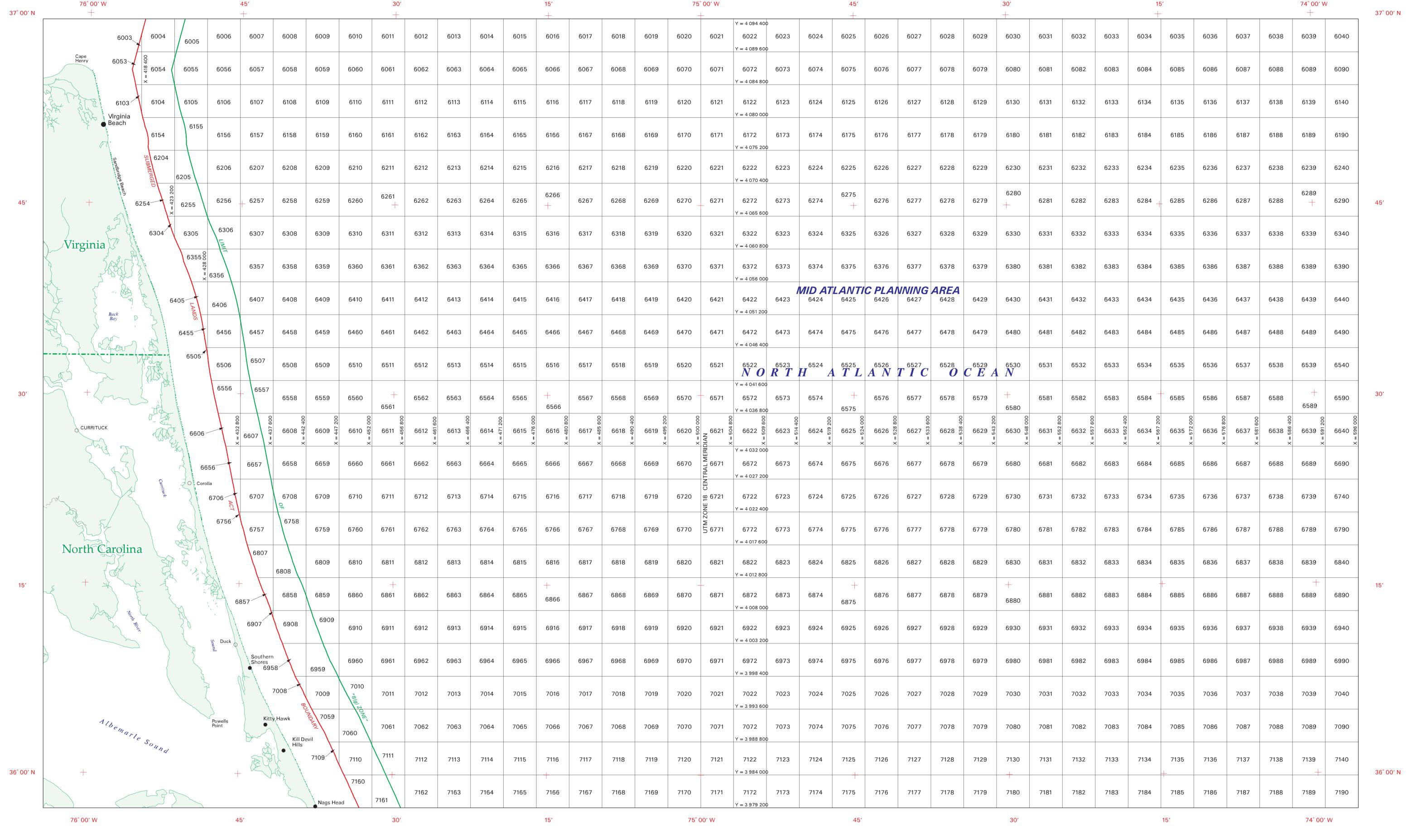
The boundaries of the regular blocks are 4,800 international meters on a side and contain 2,304 hectares. The regular boundaries are defined in terms of X and Y coordinates of the Universal Transverse Mercator Grid System based on the Geodetic Reference System (GRS) 1980 Ellipsoid.
