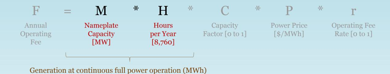
Nameplate capacity is the planned available capacity measured in megawatts (MW)
