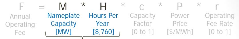
Generation at Continuous Full Power Operation [MWh]
