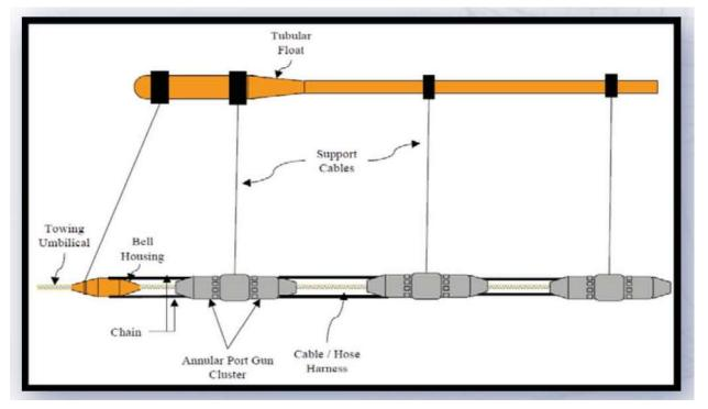
Figure 1-6. APG Sub-Array Sound Source (Example)
