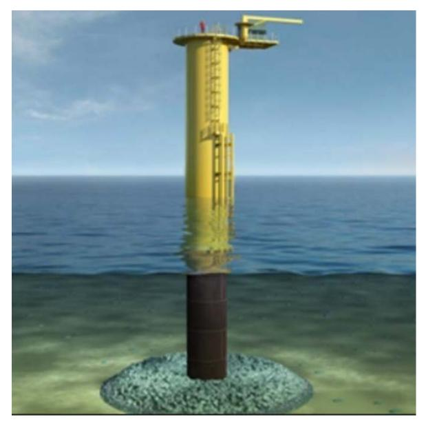
Figure 2. Illustration of monopile foundation with scour protection.
