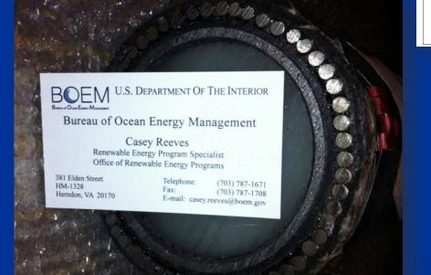
Typical 34.5-kV Submarine Transmission Cable
