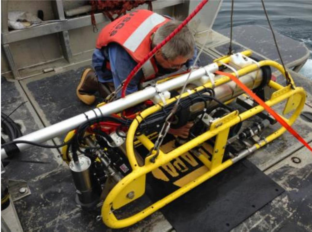
Towed high-definition video and camera sled used for groundtruthing
