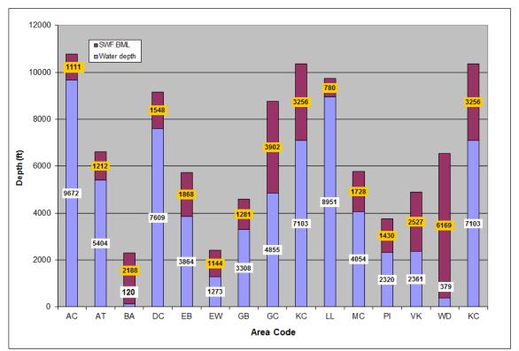
Figure 1. Average water depth and average depth BML of SWF Events
