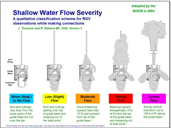
Figure 6. SWF Severity classification.
