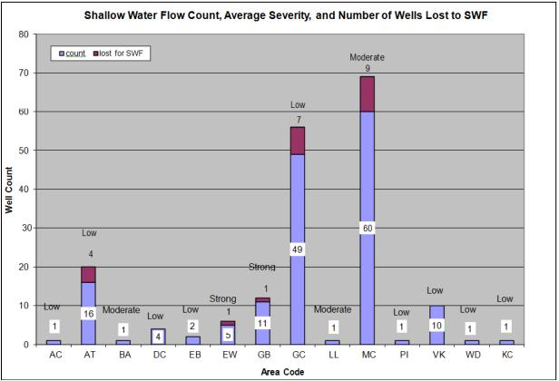
Figure 7. SWF count, average severity, and number of wells lost to SWF.
