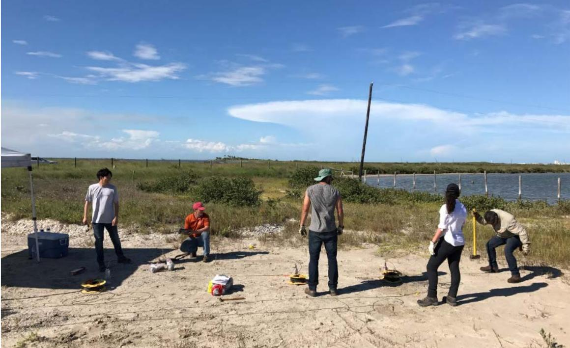
Figure 3.32 Generating waves using sledgehammer at Site 3
