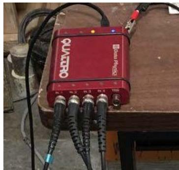
Figure 4.14 Dynamic signal analyzer (Quattro by Data Physics)
