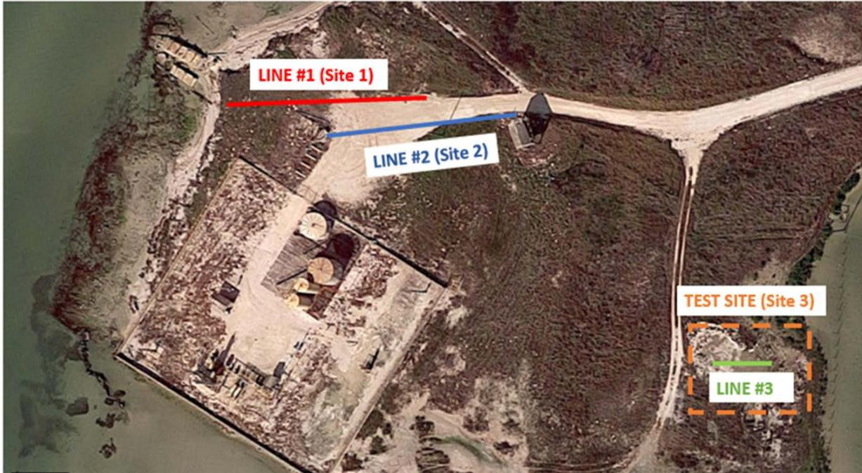
Figure 3.30 Location of the three SASW test arrays at the Mustang Island Site
