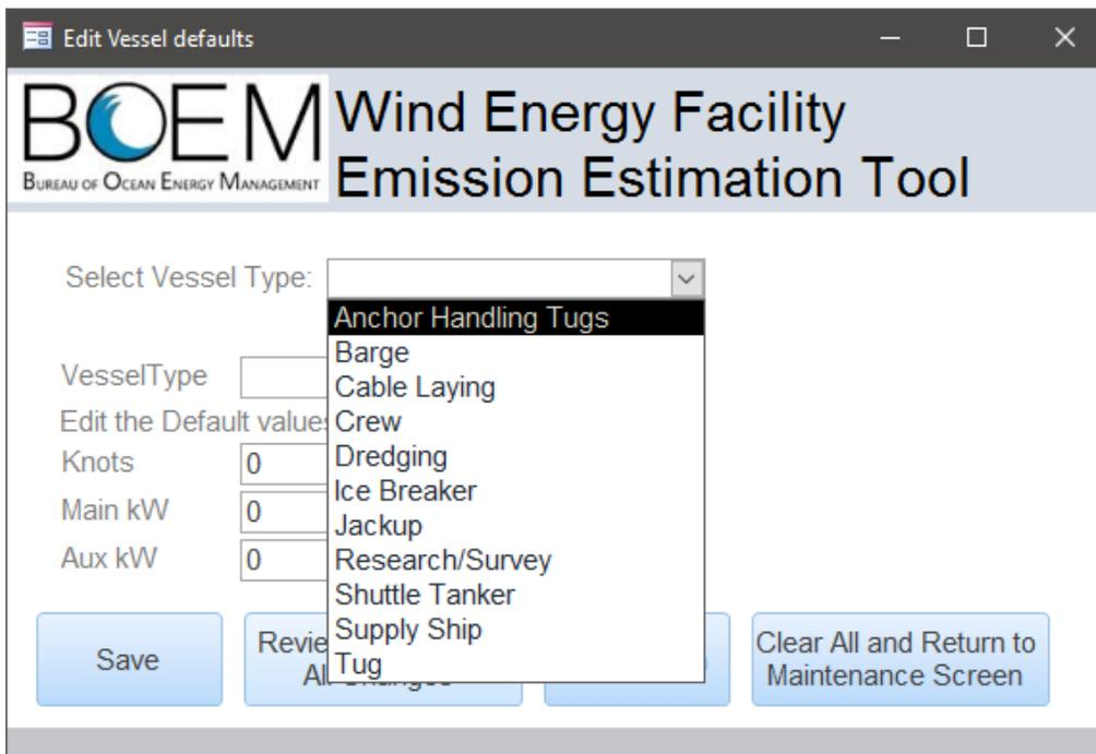
Figure 14. Vessel selection options for default edit screen
