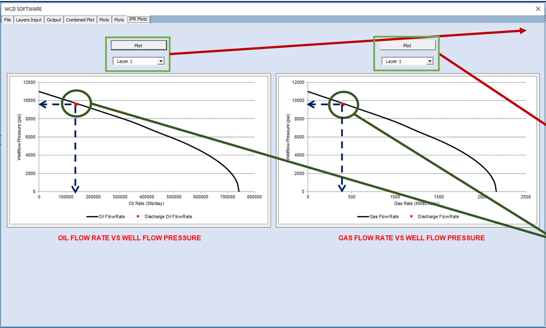
Oil flow rate Vs. Well flow pressure
