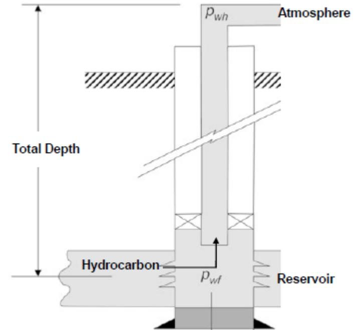
Simplified schematic of well production system (Mach et al. 1979)
