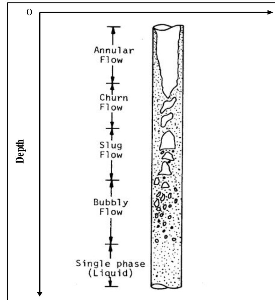
Schematic of expected two-phase flow pattern in the wellbore (Modified after Hasan and Kabir 1988)
