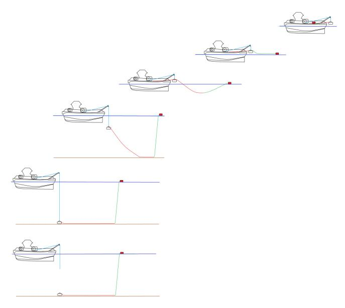
Figure 3: Diagram of riser chain deployment operation. N.B. Image is not to scale; diagram to be used as a guide to operation only. Red lines refer to chain, green lines refer to ropes, light blue lines to winch wires.
