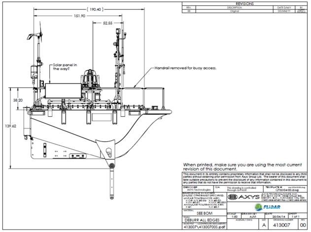
Figure 1: FLiDAR WindSentinel Dimensions – Dual ZephIR Deployment View
