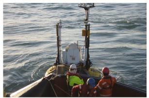
Deployment of the SEAWATCH Wind LiDAR buoy
