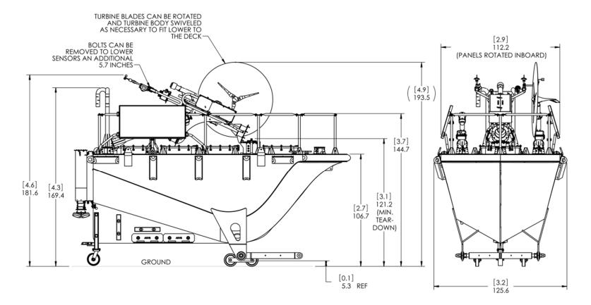
PRELIMINARY LAYOUT OF COLLAPSED WIND SENTINEL. THIS DRAWING MAY BE UPDATED PRIOR TO PROJECT COMPLETION. FINAL DESIGN (ACCESSORIES AND SENSORS) MAY NOT EXACTLY REFLECT DELIVERED SYSTEM.
