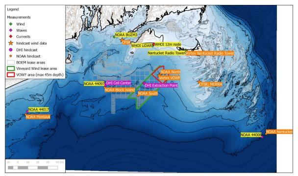
Figure 1.2.1.1: Location of the primary and secondary met-ocean data time series that were used as part of the Met-ocean analysis. Measurement locations are highlighted in yellow. Water depth contour lines are provided every 10mMSL.
