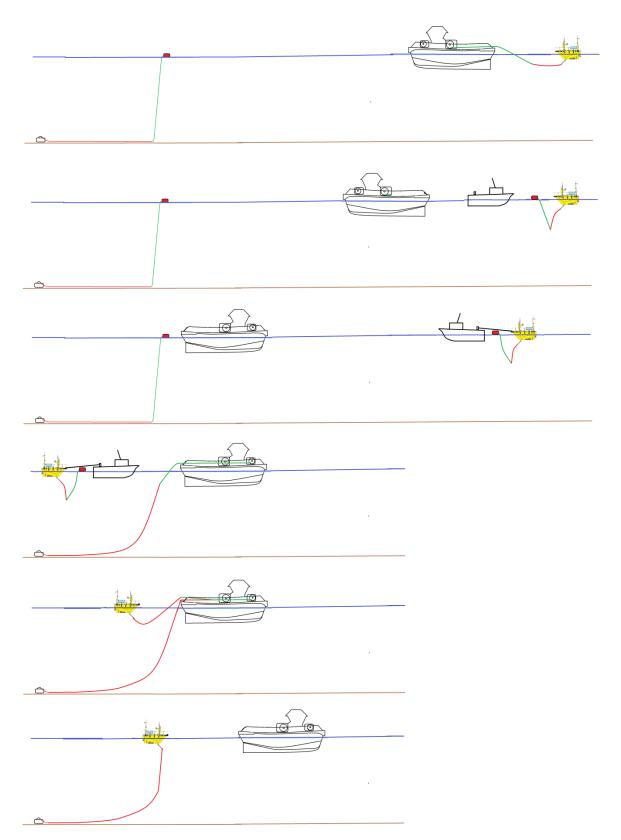
Figure 4: AXYS 6 m FLiDAR buoy deployment operations. N.B. Diagram to be used as a guide to operation only. Red lines refer to chain, green lines refer to ropes.
