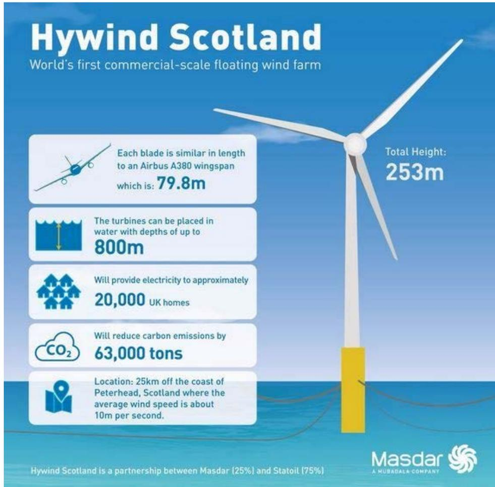
Each blade is similar in length to an Airbus A380 wingspan which is: **79.8m**
