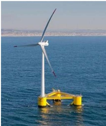
**A full-scale prototype of the WindFloat device**
