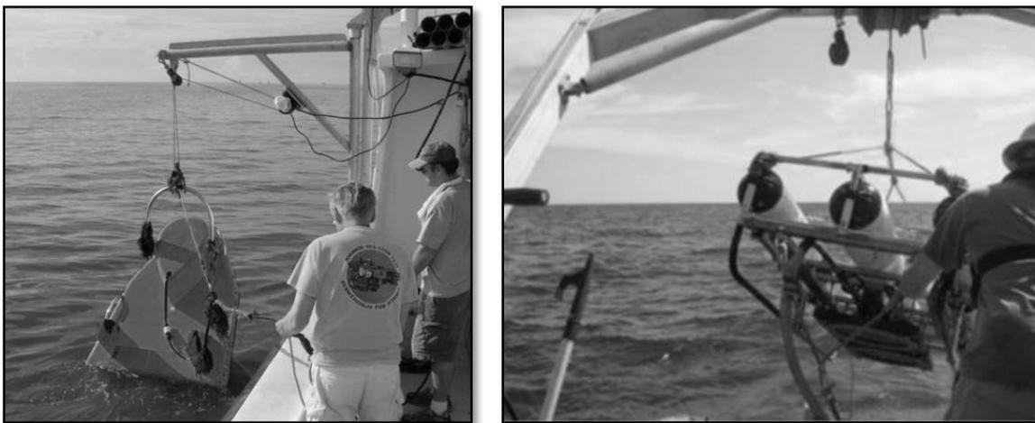
**Figure A-1. Chirp Towfish Deployment from Port (left); Boomer Sled Deployment from Stern (right)**
