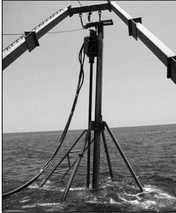
**Figure A-2. Deployment of a 20-foot Vibracore from Stern A-frame**
