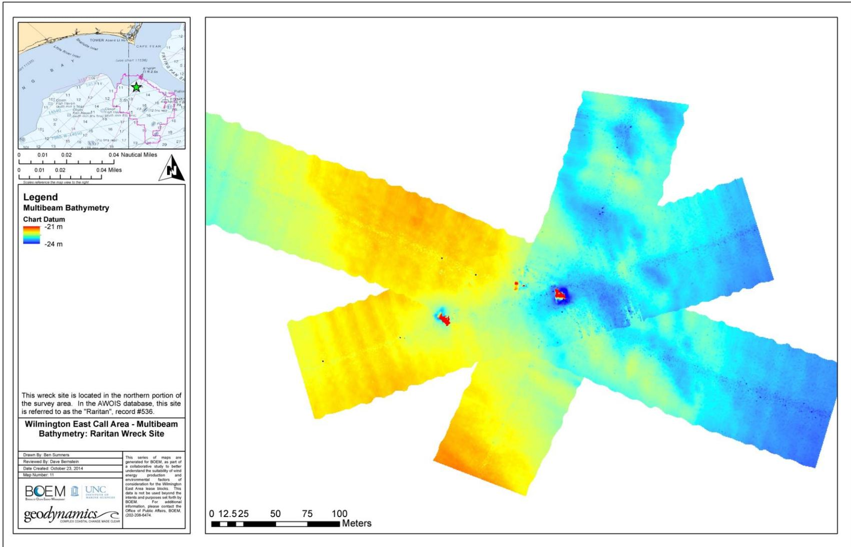
Figure 3-14. Map displaying bathymetry over the AWOIS wreck site referred to as the "Raritan".
