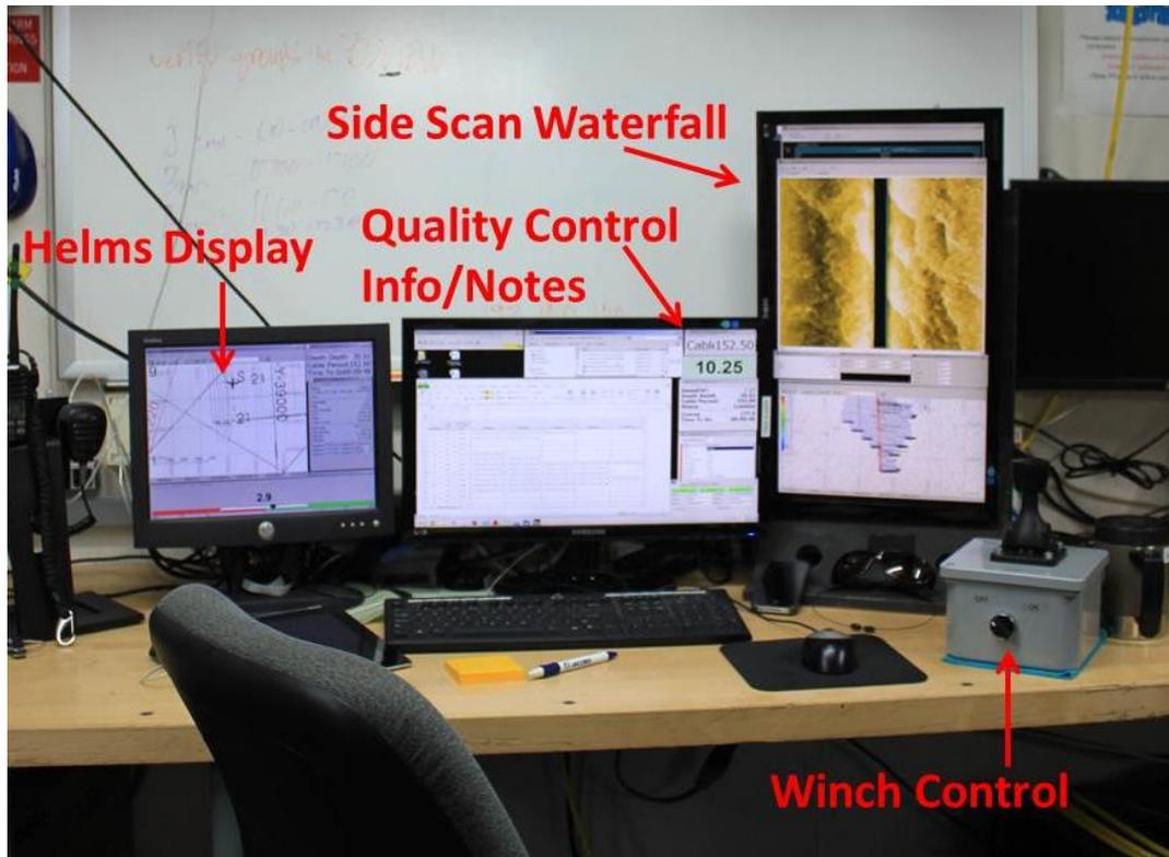
Figure 2-5. Data acquisition station for sidescan sonar operations.
