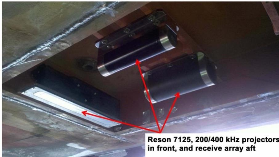
**Figure 2-3. Picture of the hull-mounted Reson 7125 transmit/receive array.**
