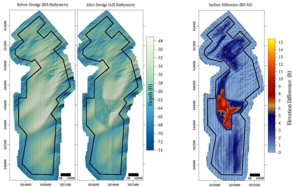
**Elevation changes in borrow area showing OCS sand removed. (Left) Seafloor condition before dredging (Spring 2017) and after dredging (Fall 2017). Dredge tracklines are visible if the after-dredge (AD) map, most clearly in the central region of the borrow area. (Right)**
