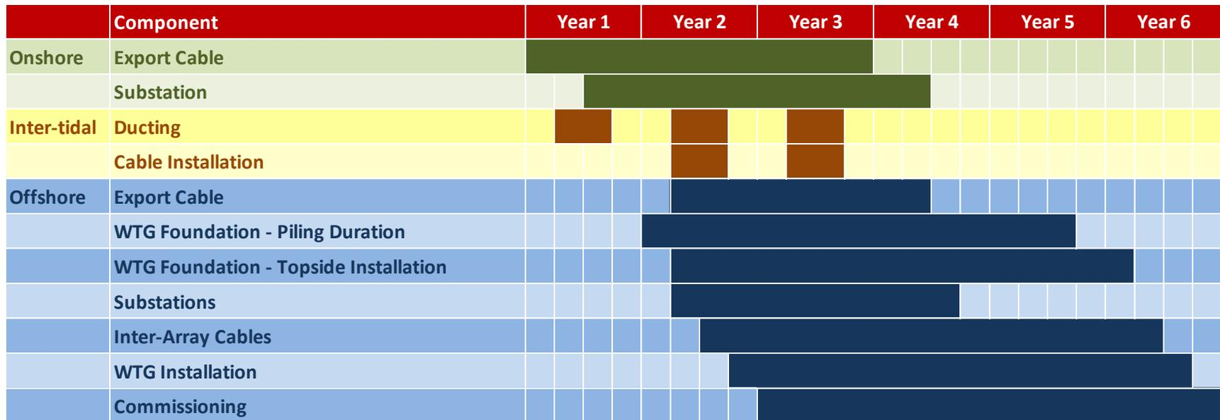
Figure B-7. Indicative Single Phased Construction Program for Hornsea Project Two.
