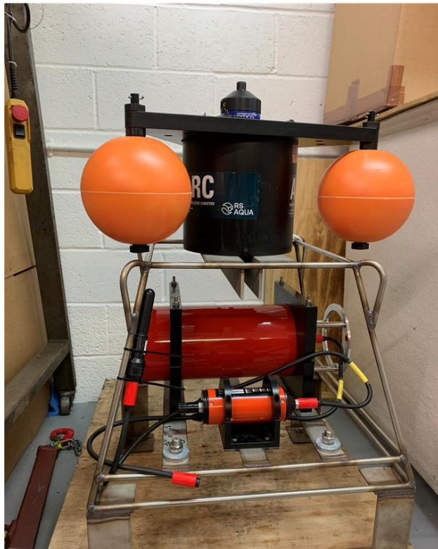
Figure 3. Example of a multi channel hydrophone array measuring 2m x 2m and weighing ~150kg
