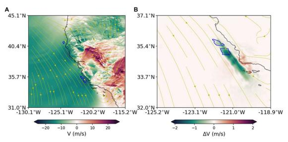
**Figure 1**. (A) Hub-height wind field on 15 Apr 2000; and (B) change in wind wake (green) due to one scenario of future wind farms. Note the O(1-2 m/s) wind speed reduction behind the Morro Bay wind energy area of interest, which would potentially reduce upwelling. From Raghukumar et al. (2022).
