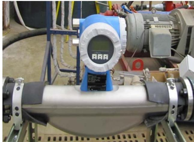
**Figure 3.6 Coriolis flowmeter**
