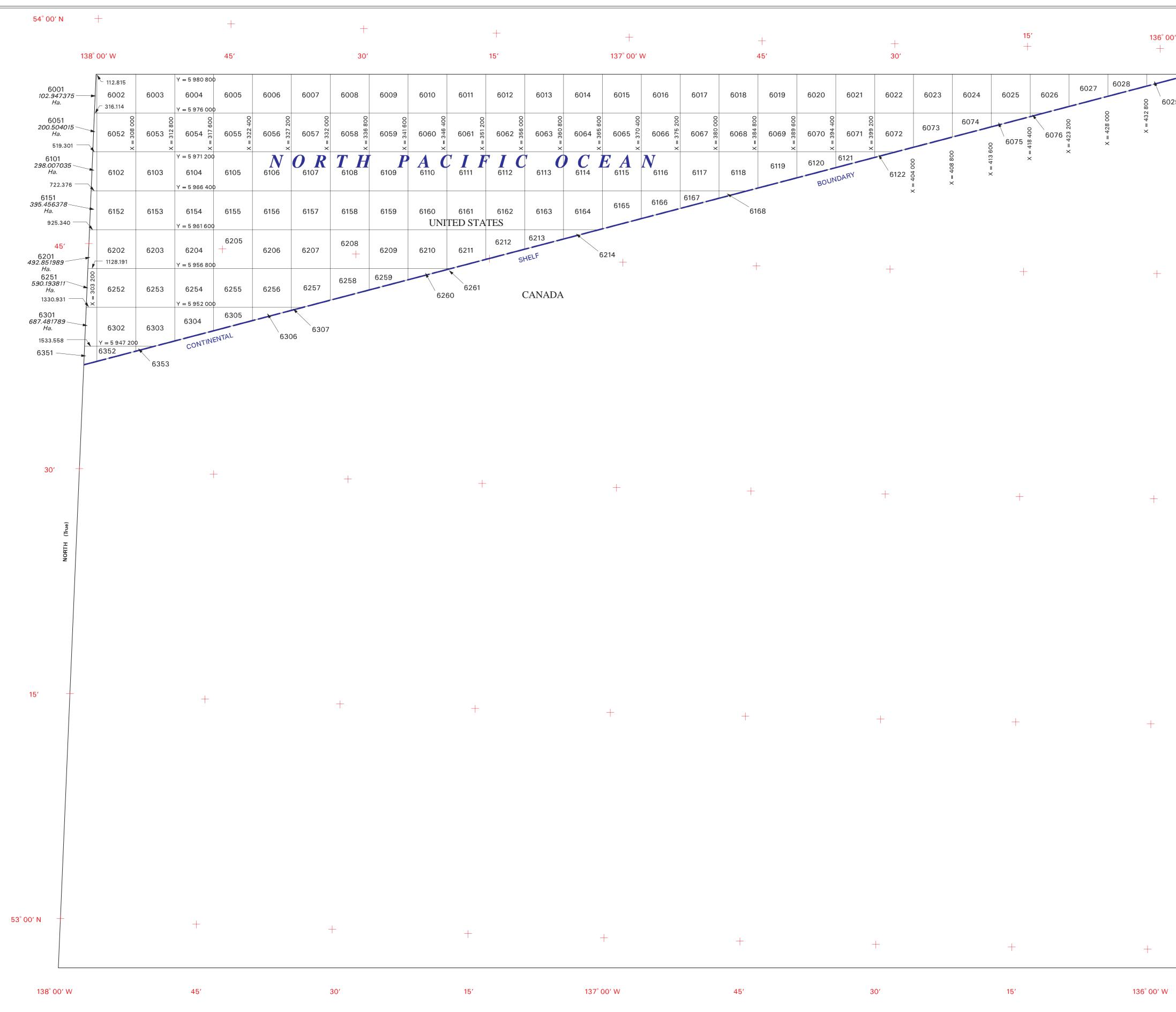
The boundaries of the regular blocks are 4,800 international meters on a side and contain 2,304 hectares. The regular boundaries are defined in terms of X and Y coordinates of the Universal Transverse Mercator Grid System based on the Geodetic Reference System (GRS) 1980 Ellipsoid.
