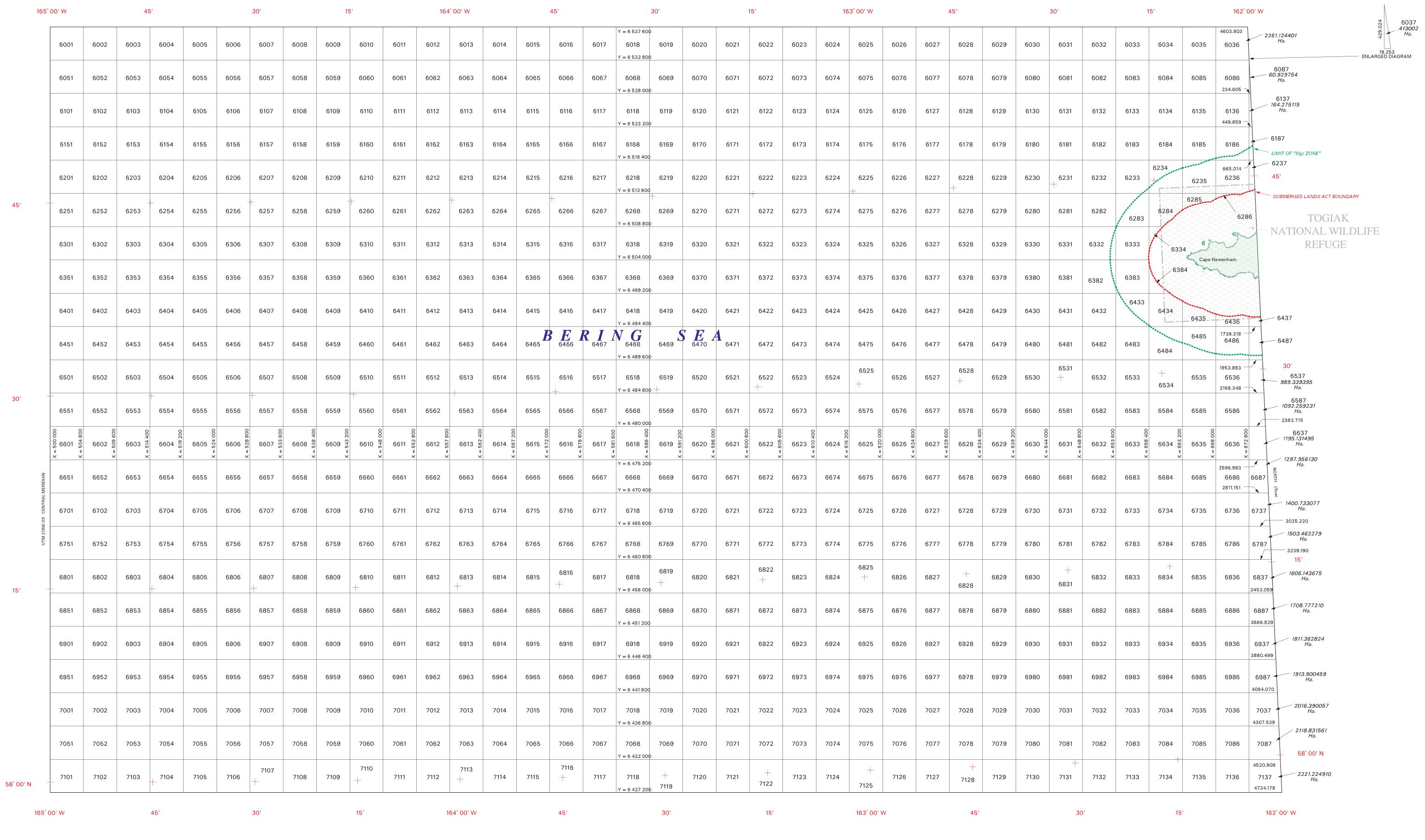
The boundaries of the regular blocks are 4,800 international meters on a side and contain 2,304 hectares. The regular boundaries are defined in terms of X and Y coordinates of the Universal Transverse Mercator Grid System based on the Geodetic Reference System (GRS) 1980 Ellipsoid.
