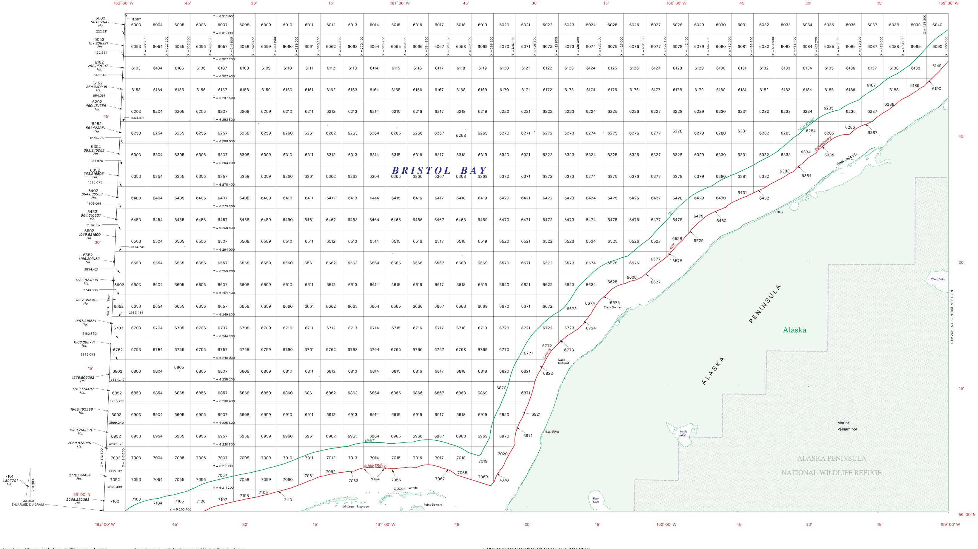
The boundaries of the regular blocks are 4,800 international meters on a side and contain 2,304 hectares. The regular boundaries are defined in terms of X and Y coordinates of the Universal Transverse Mercator Grid System based on the Geodetic Reference System (GRS) 1980 Ellipsoid.
