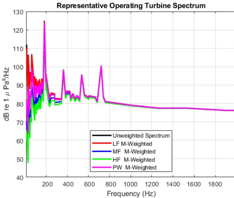
**Figure 5. Representative spectrum measured from an operating monopile turbine (from Ingemansson Technology AB, 2003).**
