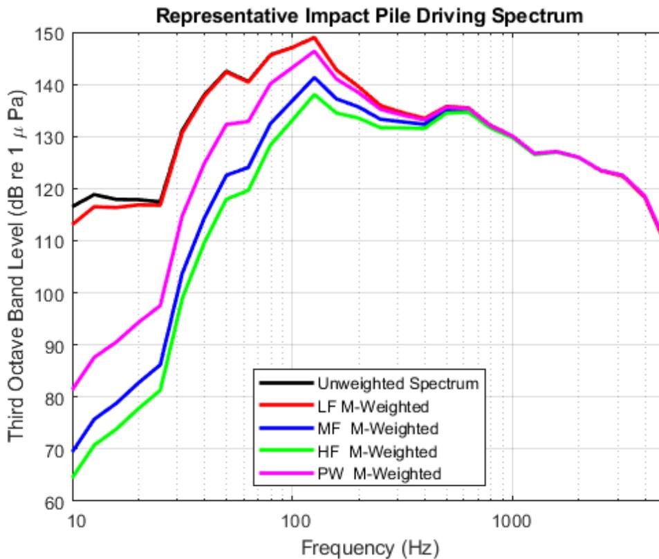
**Figure 4. Representative spectrum measured from impact pile driving of a 7.8 m monopile**
