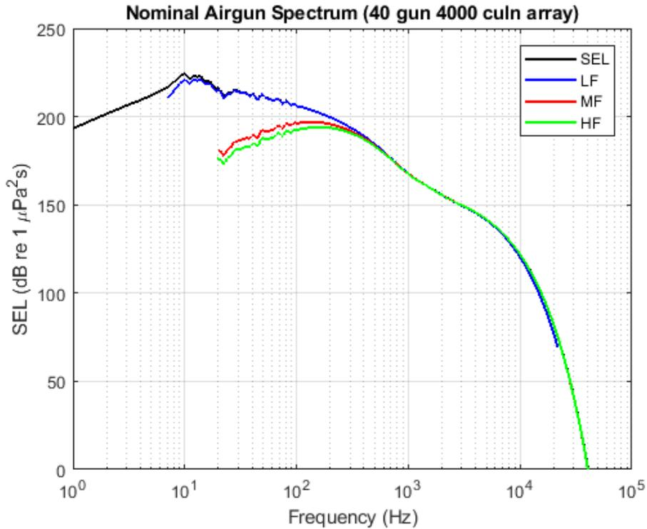
**Figure 3. Unweighted airgun spectrum (black line) compared to the spectrum weighted for LF, MF, and HF species using M-weighting**
