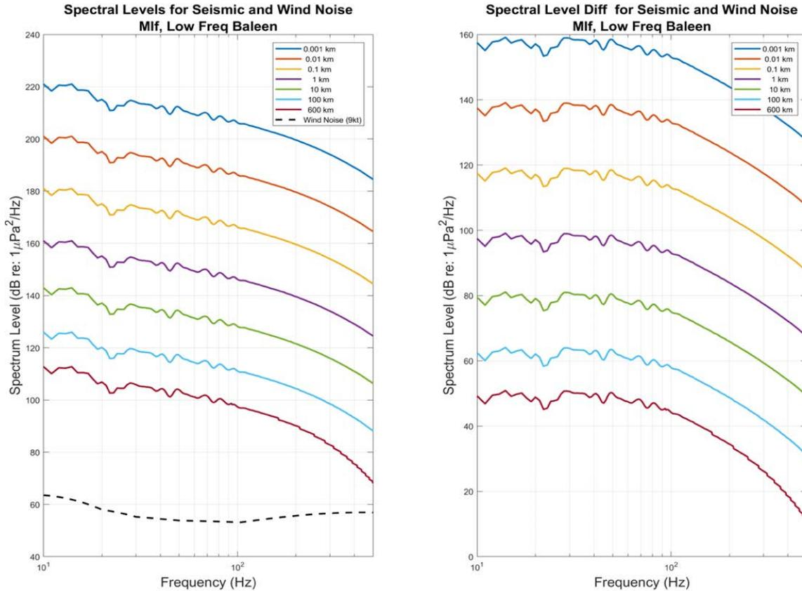
**Figure A-61B. Low-frequency, M-weighted ( $M_{lf}$ ) spectrum levels (left) for a seismic source at different distances from the source (colored lines) and spectrum level for 9 kt ambient wind noise (dashed line) and low-frequency, M-weighted ( $M_{lf}$ ) spectral differences between seismic and ambient noise spectrum levels (right).**
