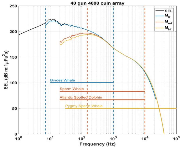
**Figure A-60. Different sound spectrum levels for a nominal spectral distribution from a 4,000 in<sup>3</sup> seismic airgun array explosion (black) after the application of the M-weighting functions for low-frequency (M<sub>lf</sub>, blue), mid-frequency (M<sub>mf</sub>, orange), and high-frequency (M<sub>hf</sub>, yellow) cetaceans.<sup>4</sup>**
