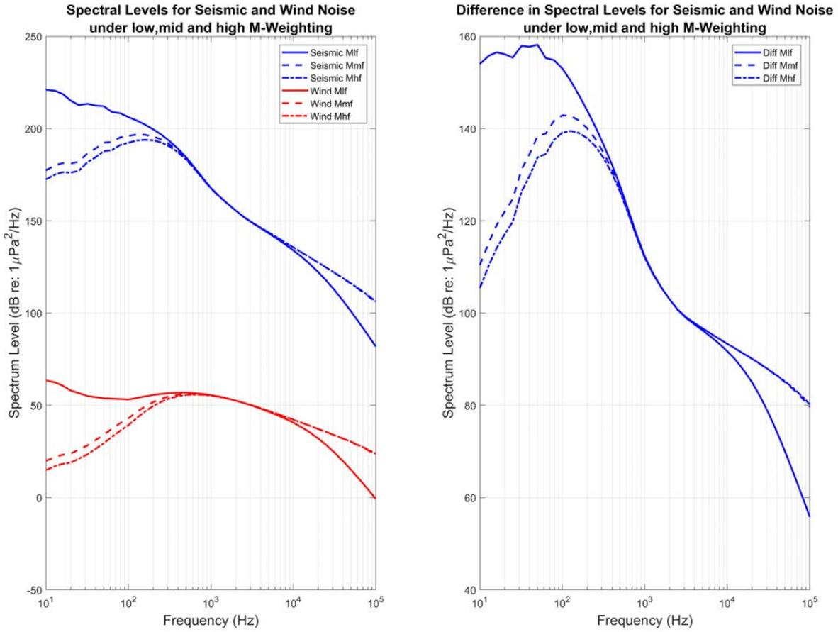
**Figure A-61A. Source spectrum levels for seismic and spectrum levels for ambient wind noise (9 kt) for each of the three M-weighted types (left) and M-weighted differences between these seismic and ambient noise spectrum levels (right).**
